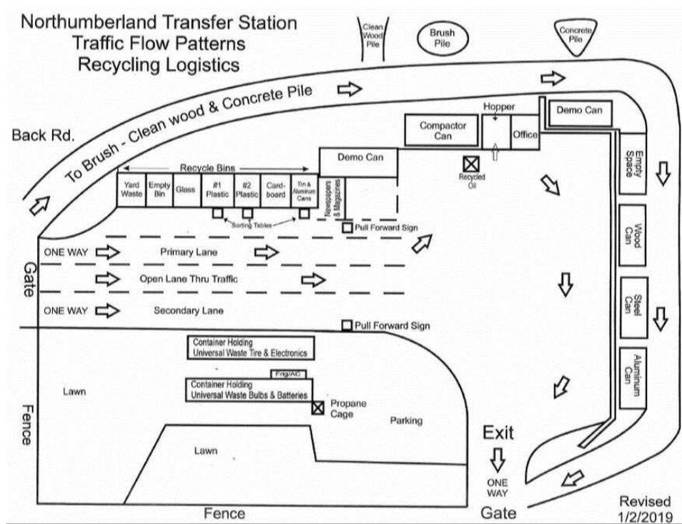
Fig. 5. Sample for transfer station traffic flow patterns [18].
