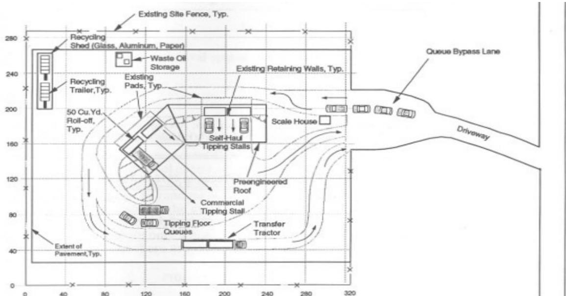
Fig. 4. Conceptual level design of Riley County Transfer Station for small site [17].
