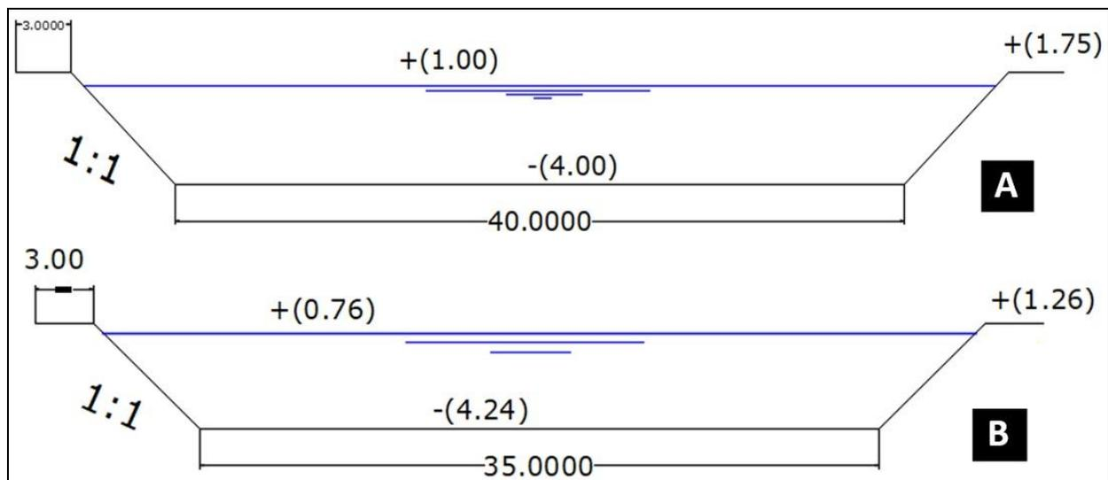
**Fig. 13.** Designed parameters of cross-sections A) No. 1 just downstream of El-Max Pump Station km (1.010); and B) No. 102 at the mouth of the drain-reach km (0.000) for a maximum discharge of 195 m<sup>3</sup>/sec.
