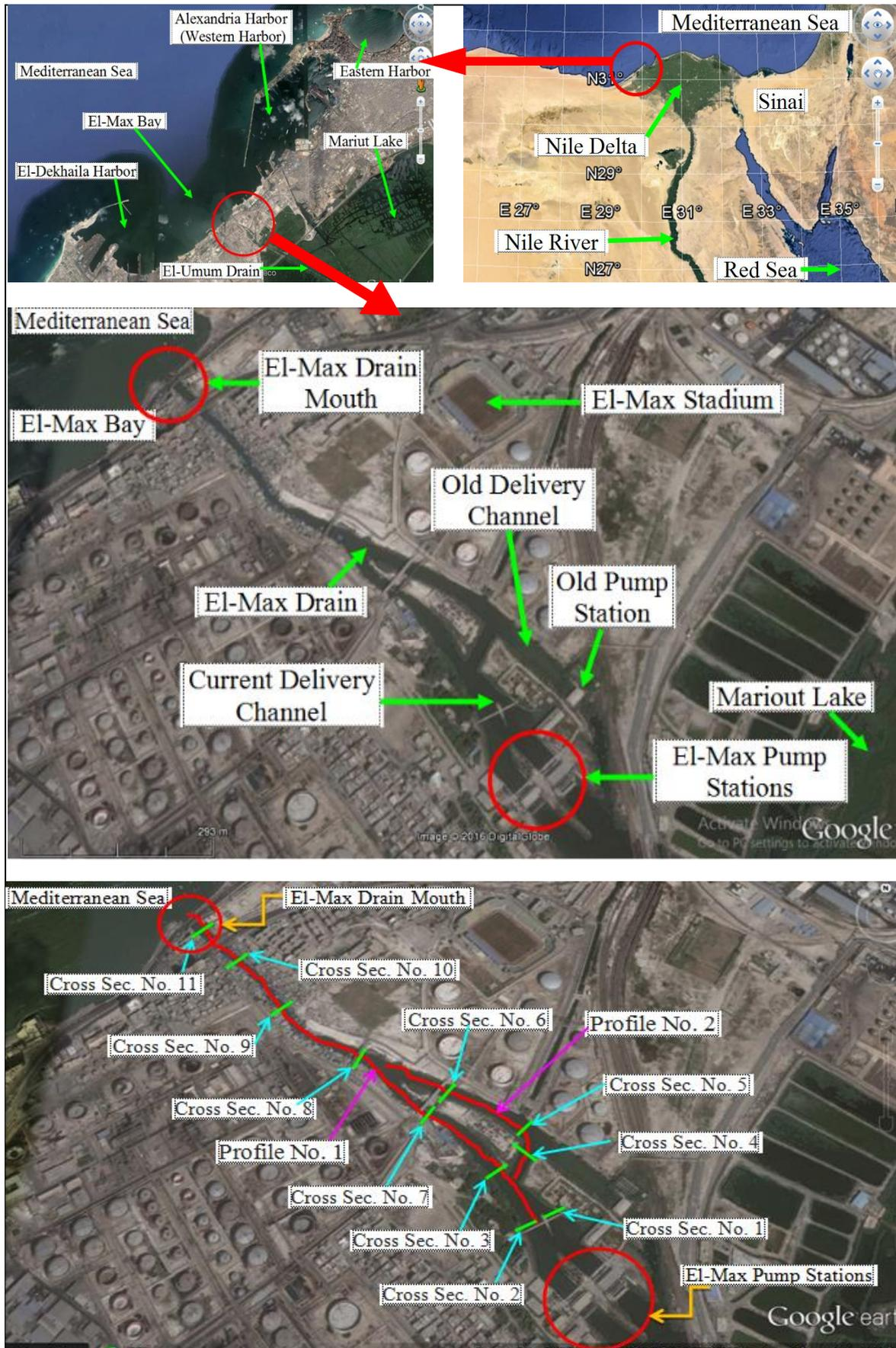
Fig. 1. Google Earth satellite image showing the general layout of El-Max Pump Stations and hydrographic survey profiles of the drain mouth on the Mediterranean Sea on 6<sup>th</sup> January 2016 [1].
