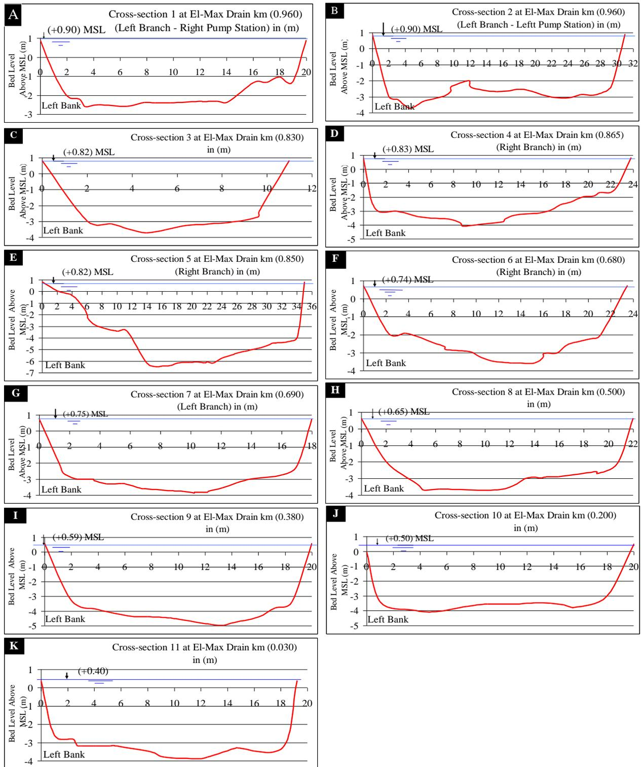
Fig. 8. Cross-sections 1, 2, 3, 4, 5, 6, 7, 8, 9, 10 and 11 at the drain-reach on 6<sup>th</sup> January 2016 [1].
