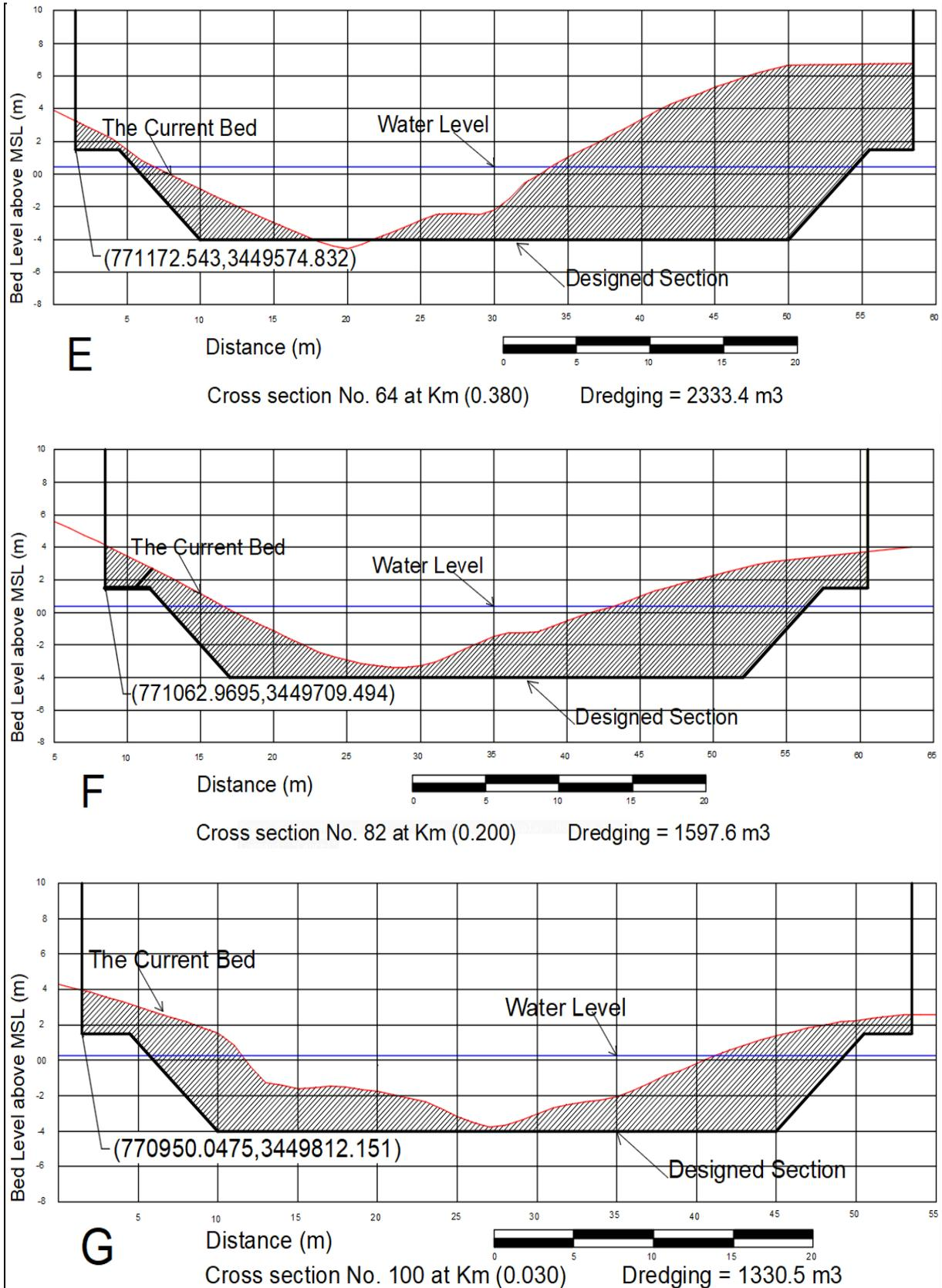
Fig. 12B. Cross-sections 64, 82, and 100 at the drain-reach on 13<sup>th</sup> October 2016.
