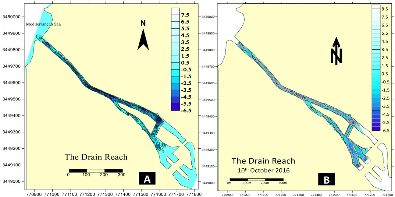
Fig. 9. Contour map of the study area (Bathymetry) A) on 6<sup>th</sup> January 2016, and B) on 13<sup>rd</sup> October 2016.
