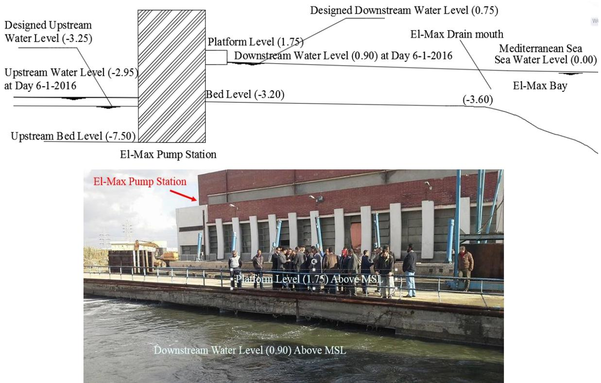
Fig. 2. Parameters schematic diagram, the platform just downstream of El-Max Pump Stations and the Drain Reach mouth on 6<sup>th</sup> January 2016 [1].
