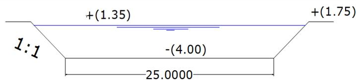
Fig. 11. Water surface for all scenarios in the hydraulic model operating and the designed parameters of cross-section No. 1 just downstream of El-Max Pump Station km (1.010) for a maximum discharge of 174.5 m<sup>3</sup>/sec. [1].
