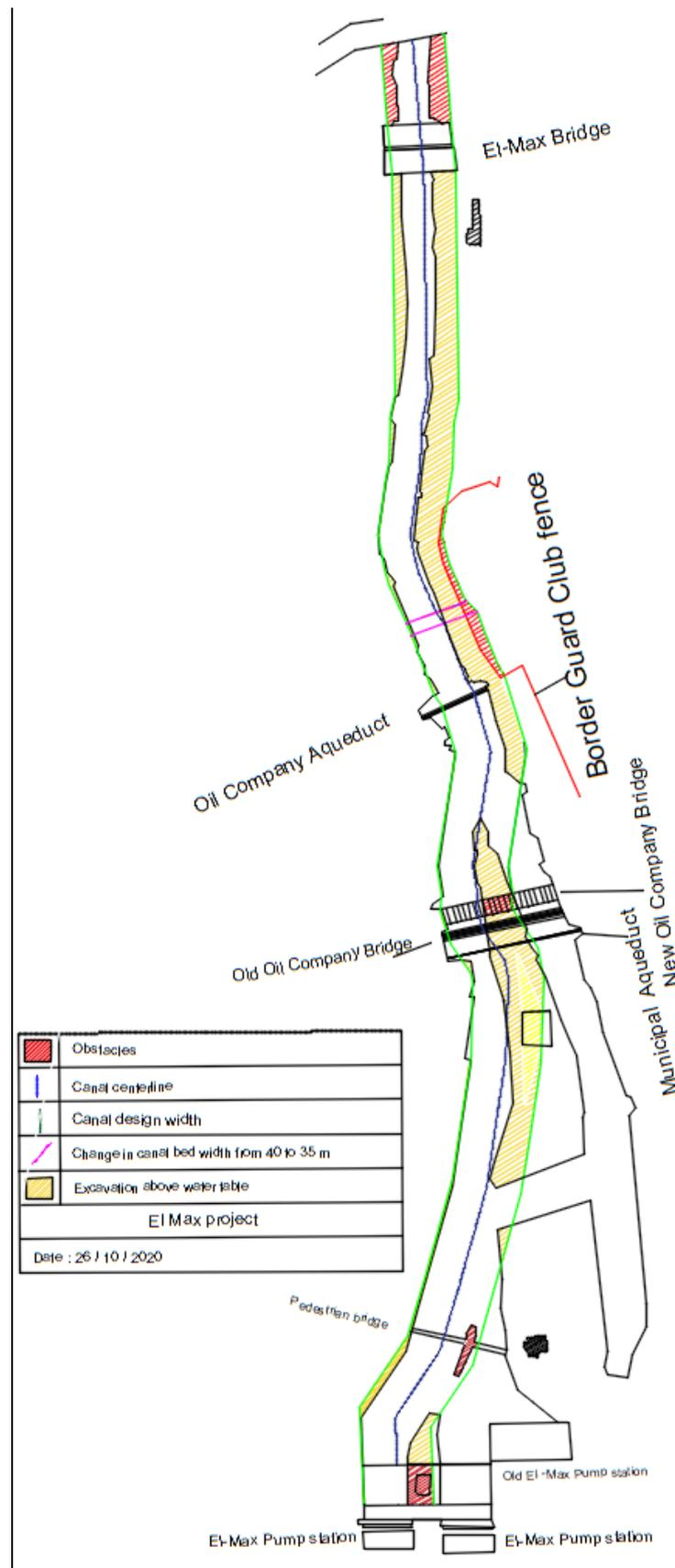
**Fig. 15.** The layout of the drain reach and the newly designed plan for the dashed areas to dredge, the obstacles in implementation, and objections to the bases and foundations of the bridges of the oil companies inside the drain path.
