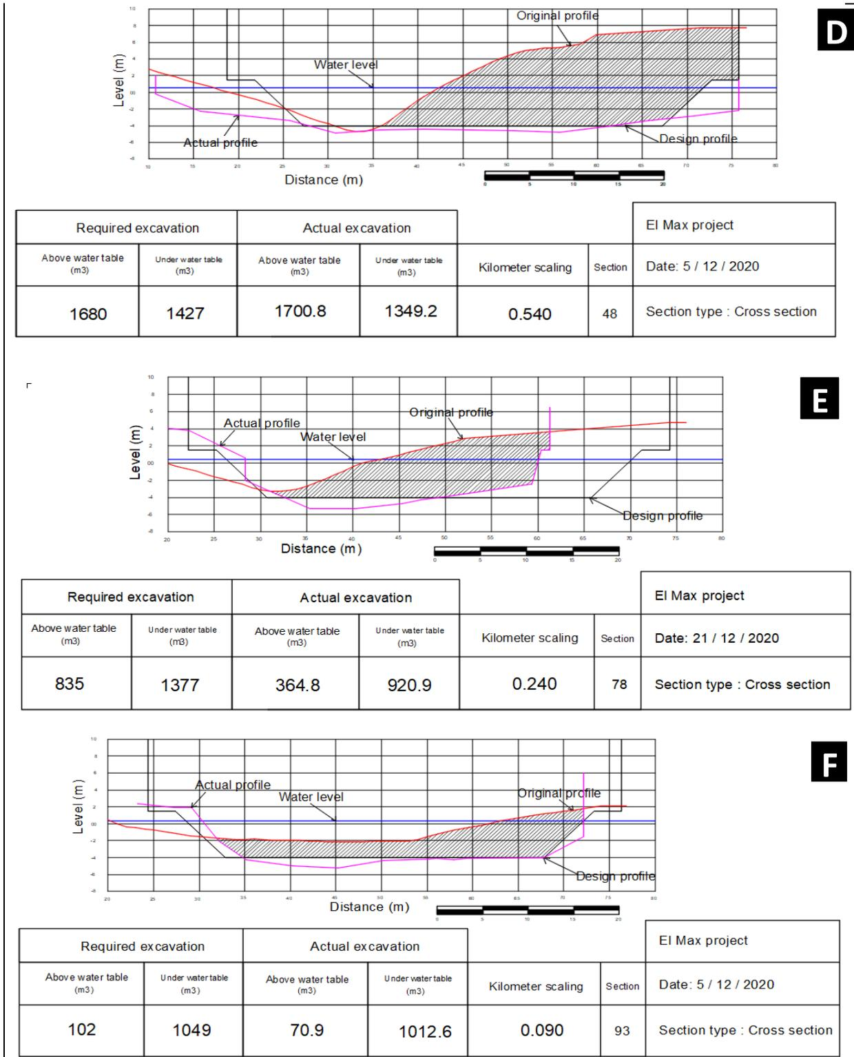
Fig. 17. The bed levels for actual profiles in December 2020, original profiles measured on the 13<sup>th</sup> of 2016, and the newly designed sections D) Profile 38; E) Profile 78; and F) Profile 93.
