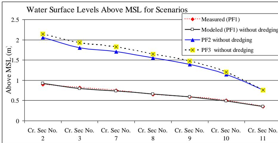
Fig. 10. Water surface calibration between measured and modeled values for 6<sup>th</sup> Jan. 2016 for PF1 scenario and scenarios without dredging [1].
