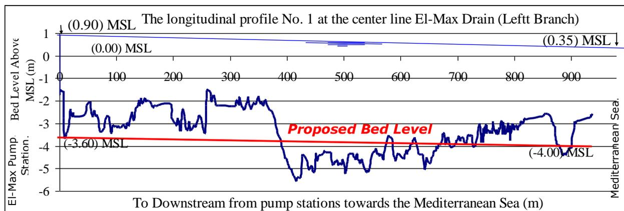
**Fig. 7.** Longitudinal profile 1 at the center line of the drain-reach (left branch) on 6<sup>th</sup> January 2016 [1].
