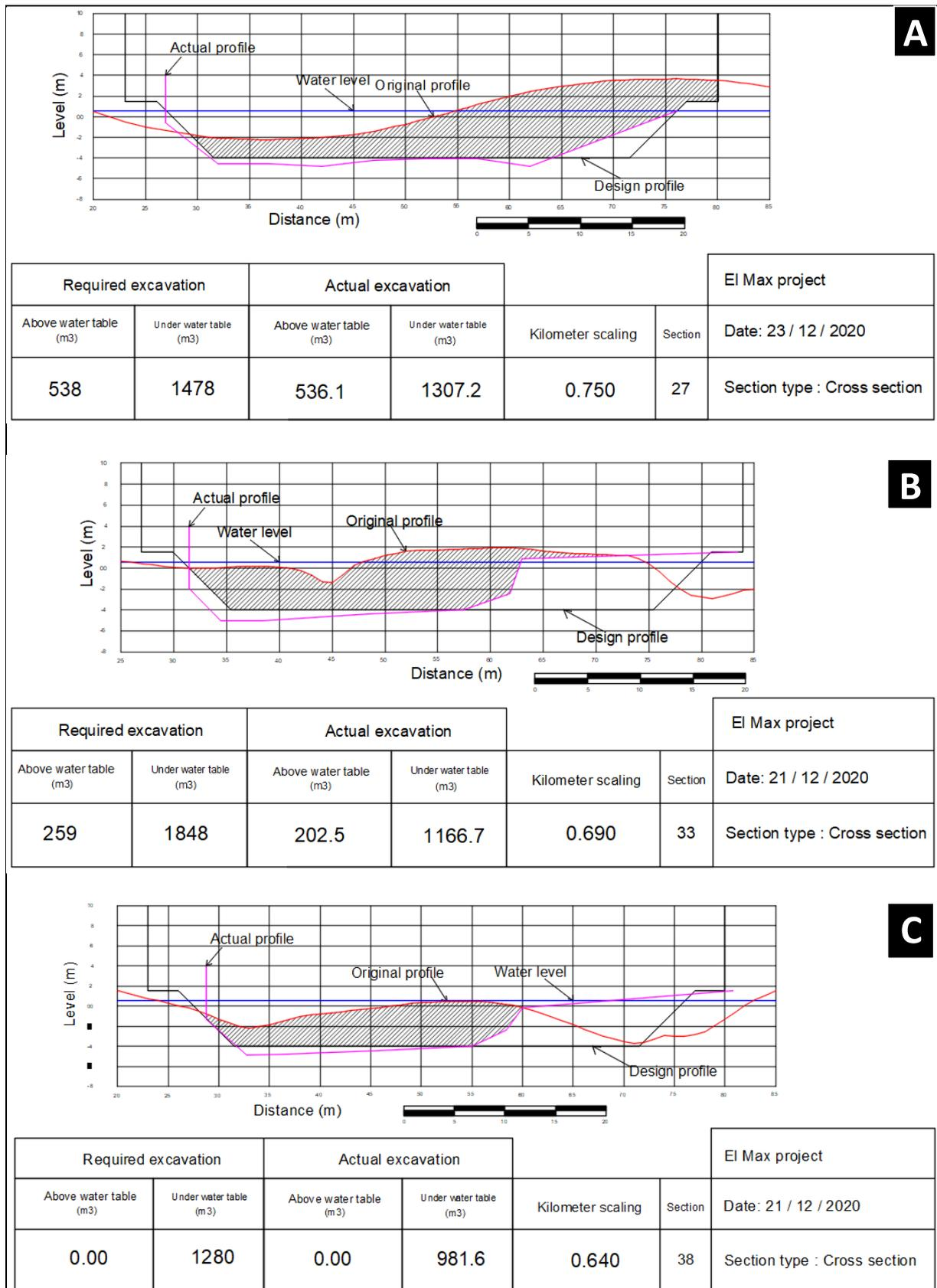
Fig. 16. The bed levels for actual profiles in December 2020, original profiles measured on the 13<sup>th</sup> of 2016, and the newly designed sections A) Profile 27; B) Profile 33; and C) Profile 38.
