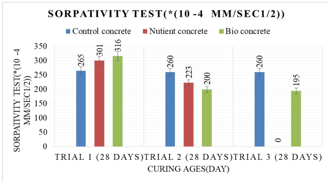
Fig. 13. Charts the sorpativity test results for hardened concrete in three trial mix.
