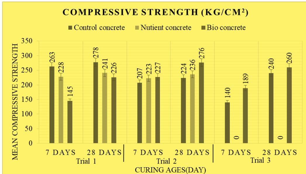
**Fig. 10.** Charts the compressive strength test results for hardened concrete in three trial mix.
