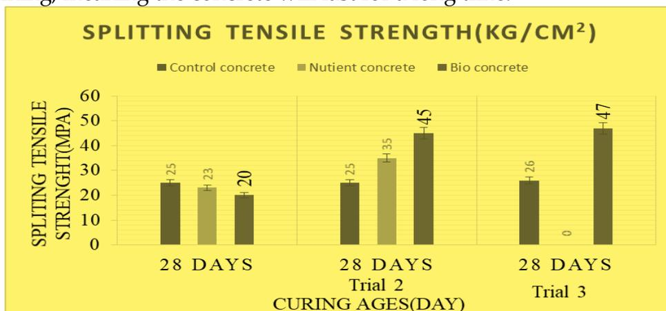
Fig. 12. Charts the Tensile strength splitting testing results for hardened concrete in three trial mix.
