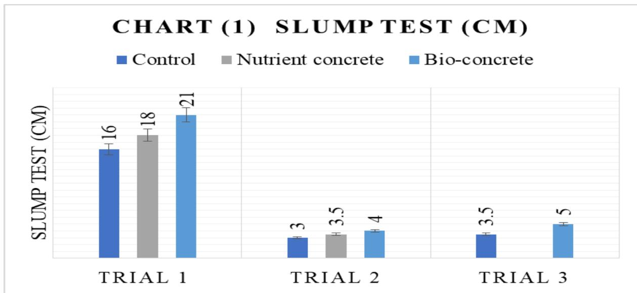
Fig. 9. Charts the slump test results for fresh concrete in three trial mix.
