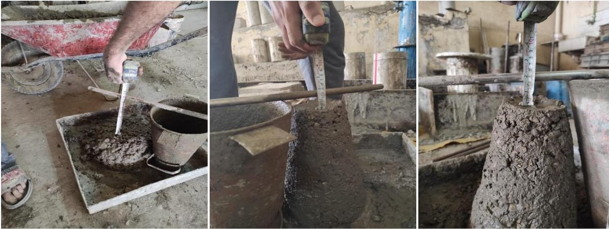
Fig. 8. Some pictures of three mixtures for concrete Slump of fresh concrete.
