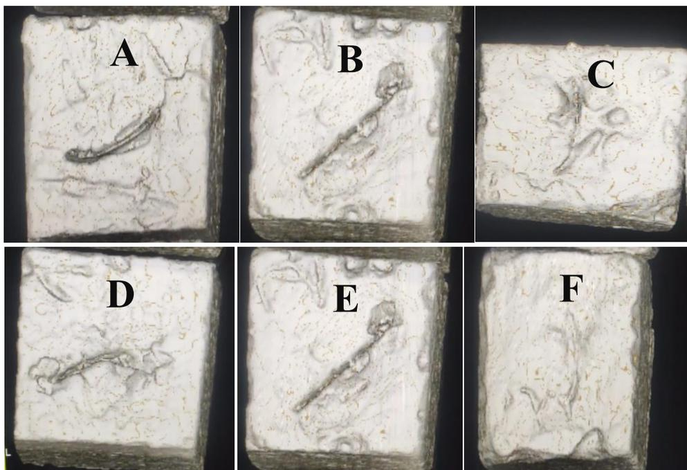
Fig. 14. X rays CT test for Concrete sample from 2 trial mix where: (A and D) Control concrete, (B and E) Nutrient concrete and (C and F) Bio concrete.
