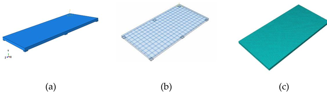
**Fig. 1.** (a) FE Model, (b) Reinforcement and (c) Mesh Layout used for the Slab.
