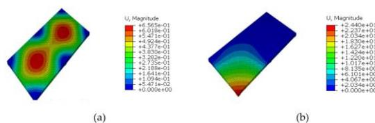
**Fig. 3.** Deformed Profile of the Slab (a) Before Column Removal and (b) After Column Removal.
