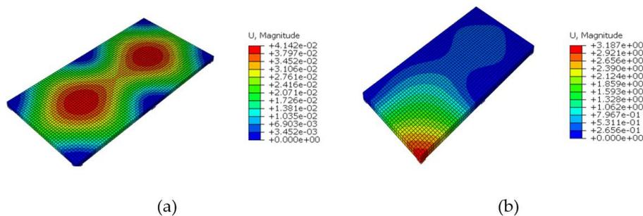
**Fig. 9.** Deformed Profile of Slab having Thickness of 125mm (Case Study-C125) (a) Before Column Removal and (b) After Column Removal.
