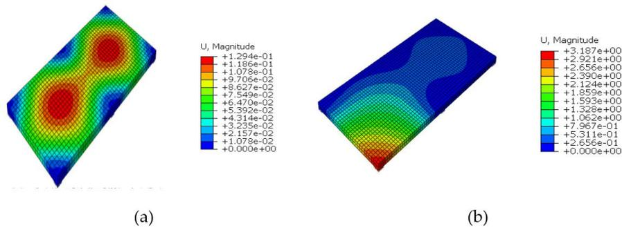
**Fig. 10.** Deformed Profile of Slab having Thickness of 160mm (Case Study-C160) (a) Before Column Removal and (b) After Column Removal.
