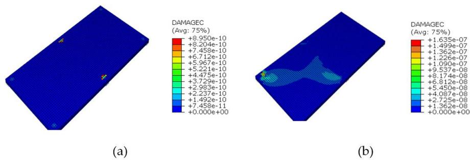
**Fig. 4.** Damage Caused to the Slab in Terms of Compression Crushing (a) Before Column Removal and (b) After Column Removal.
