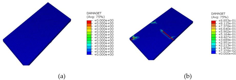
**Fig. 5.** Damage Caused to the Slab in Terms of Tensile Cracking (a) Before Column Removal and (b) After Column Removal.
