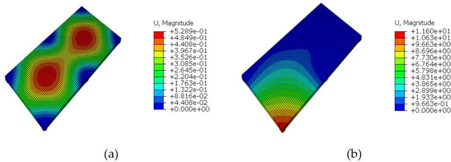
**Fig. 6.** Deformed Profile of the Slab used in Case Study-C40 (a) Before Column Removal and (b) After Column Removal.
