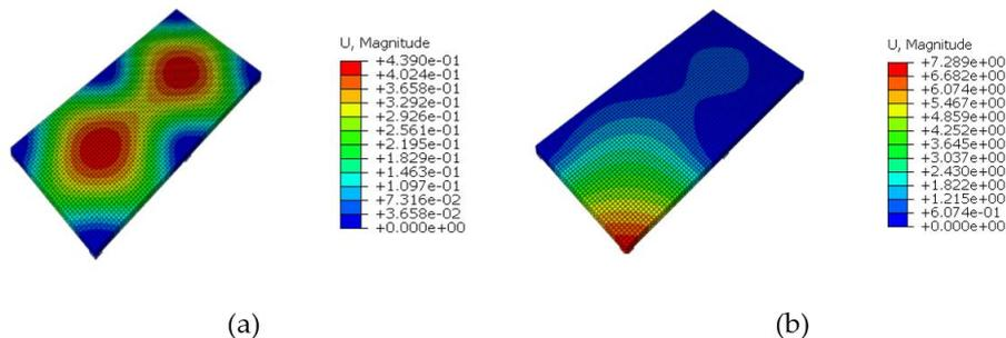
**Fig. 7.** Deformed Profile of the Slab used in Case Study-C60 (a) Before Column Removal and (b) After Column Removal.
