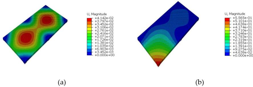
**Fig. 8.** Deformed Profile of the Slab used in Case Study-C80 (a) Before Column Removal and (b) After Column Removal.
