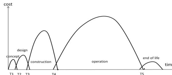
**Fig. 4:** Project Main Phases and Its Relation With Time And Cost
