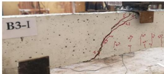
c) Crack patterns for beam B3-I
