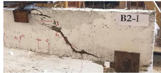
b) Crack patterns for beam B2-I
