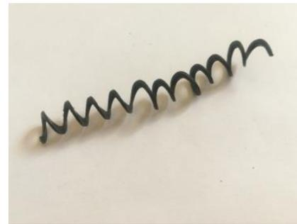
**Fig. 3.** Recycled lathe fiber shape.
