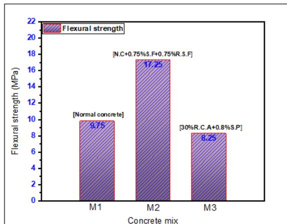
**Fig. 9.** Flexural strength for three different concrete mixes after 28 days.
