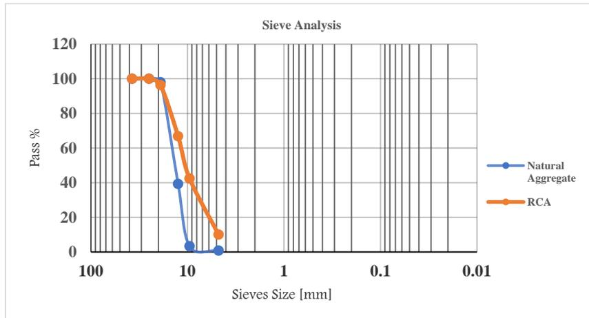
**Fig. 1.** Sieve analysis of NA and RCA.
