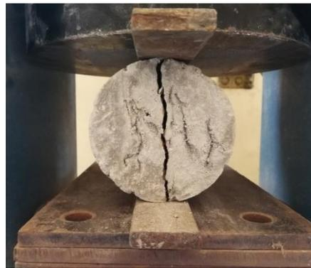
**Fig. 5.** Indirect tension test.
