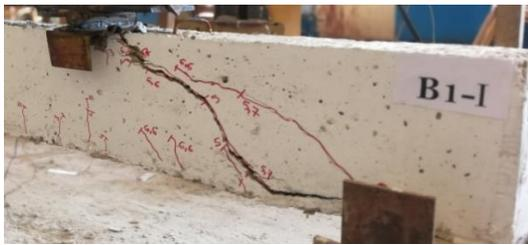
a) Crack patterns for beam B1-I
