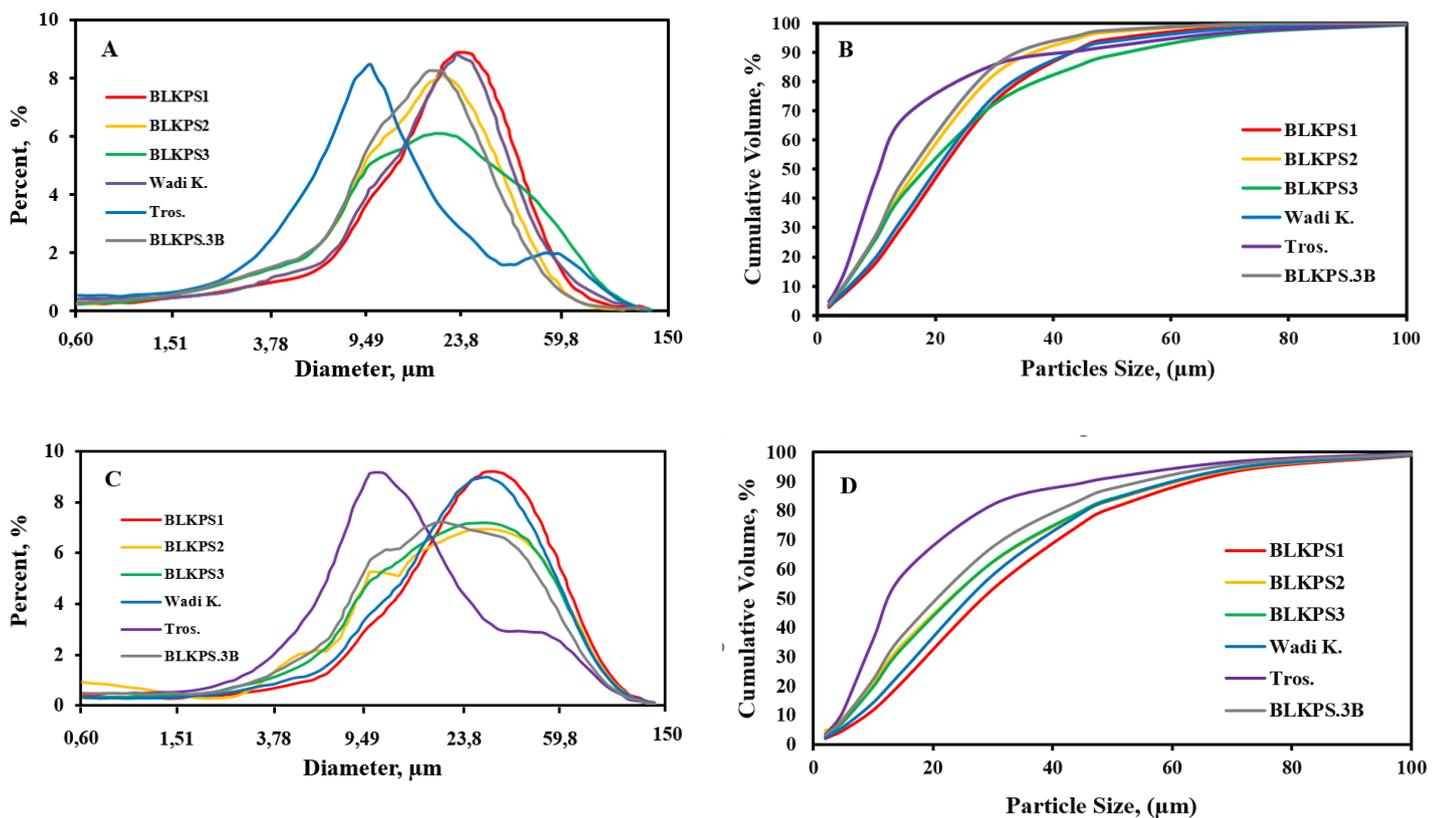
**Fig. 4.** Effect of  $\text{SiO}_2 / \text{Al}_2\text{O}_3$  ratio on the Self-disintegration process efficiency of kaolin-limestone mixture from different locations in the presence of 1.5% charcoal: (A) frequency curves and (B) cumulative curves of the sinters; (C) frequency curves and (D) cumulative curves of the related sludges obtained after the leaching process.
