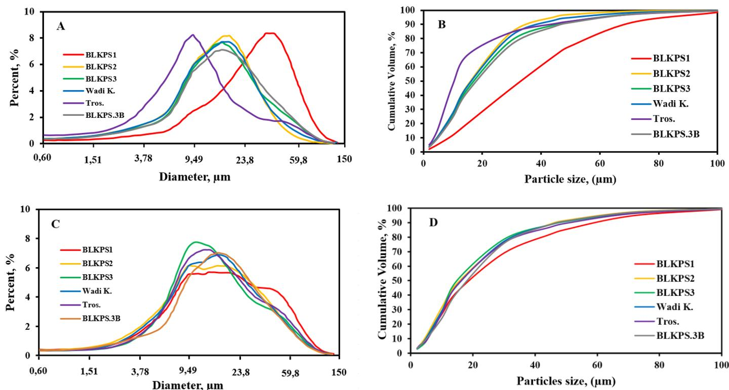
**Fig. 3.** Effect of silicate module on the efficiency of the Self-disintegration process of the sintered kaolin-limestone mixtures from different locations in the absence of charcoal addition: (A) frequency curves and (B) cumulative curves of the sinters; (C) frequency curves and (D) cumulative curves of the related sludges obtained after the leaching process.
