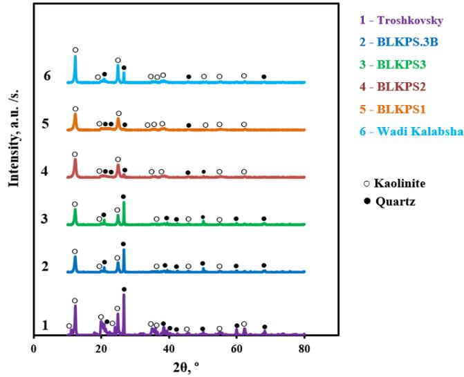
Fig. 1. X-ray diffractograms of kaolin ore samples from different locations.
