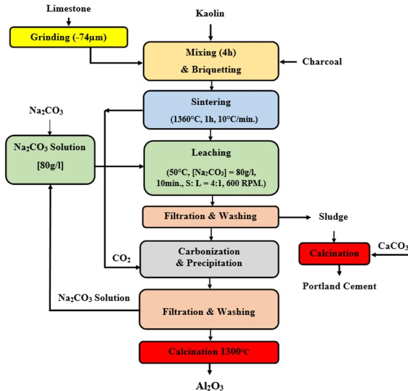
**Fig. 6.** The proposed technology for the Pyro-hydro metallurgical processing of kaolin ore using a thermo-chemically activated lime-sinter process for alumina extraction.
