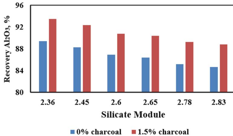
**Fig. 5.** Dependence of the  $\text{Al}_2\text{O}_3$  percent recovery from the sintered kaolin-limestone mixture on the silicate module of kaolin ore with and without the addition of charcoal at  $1360^\circ\text{C}$ .
