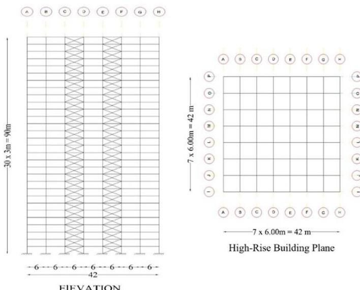
Fig.9 A 30-storey steel frame building (42x42) with Hight= 30x3.0= 90.m.
