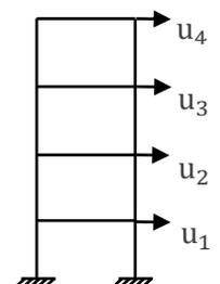
Fig.1 4-story Shear building Example [36].
