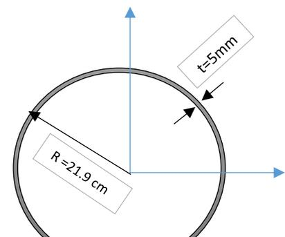
Fig. 7 Fig. 8. Pipe section  $R= 21.9$  cm &  $t=5\text{mm}$  for Bracing sections.
