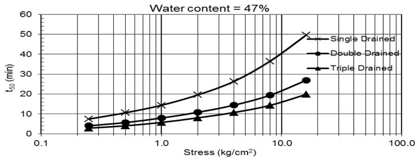
Fig. 16: Relationship between time of consolidation (T<sub>50</sub>) and stresses for different drainage at water content 47%
