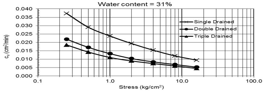
**Fig. 9: Relationship between coefficient of consolidation ( $c_v$ ) and stresses for different drainage at water content 31%**
