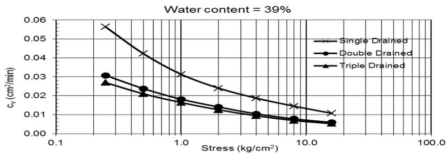
**Fig. 10: Relationship between coefficient of consolidation ( $c_v$ ) and stresses for different drainage at water content 39%**
