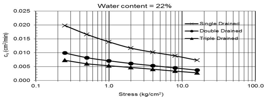
**Fig. 8: Relationship between coefficient of consolidation ( $c_v$ ) and stresses for different drainage at water content 22%**
