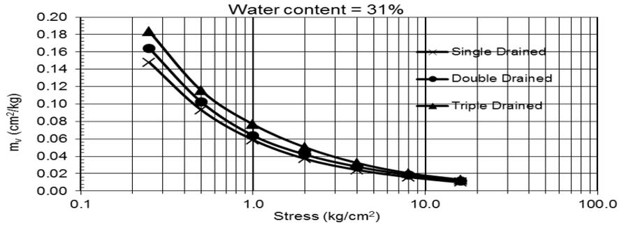
**Fig. 4: Relationship between the coefficient of volume change ( $m_v$ ) and stresses for different drainage at water content 31%**
