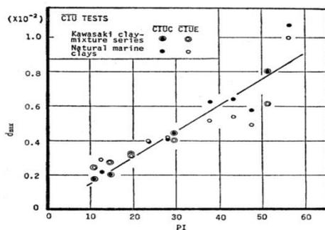
Fig. 1: Relationship between the  $d_{max}$  and PI in CIU (isotropically consolidated undrained test) tests
