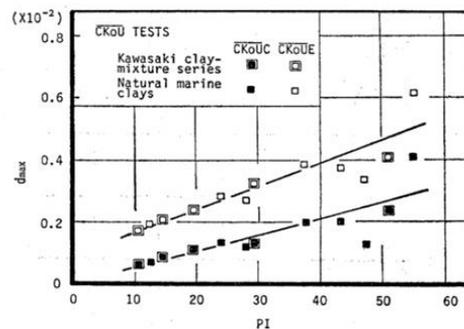
Fig. 2: Relationship between the  $d_{max}$  and PI in CKoU (consolidated undrained test) tests
