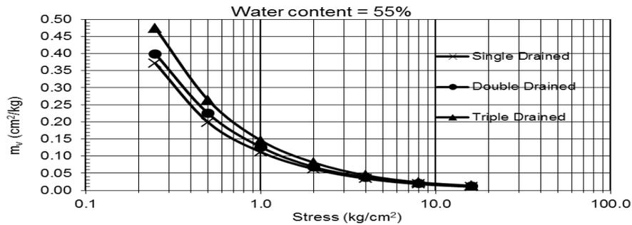
**Fig. 7: Relationship between the coefficient of volume change ( $m_v$ ) and stresses for different drainage at water content 55%**
