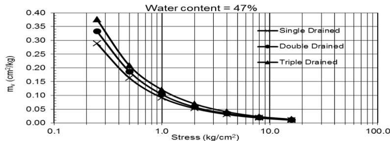
**Fig. 6: Relationship between the coefficient of volume change ( $m_v$ ) and stresses for different drainage at water content 47%**
