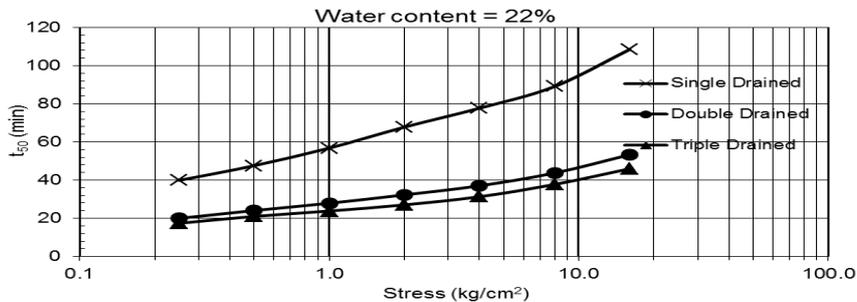
Fig. 13: Relationship between time of consolidation ( $t_{50}$ ) and stresses for different drainage at water content 22%
