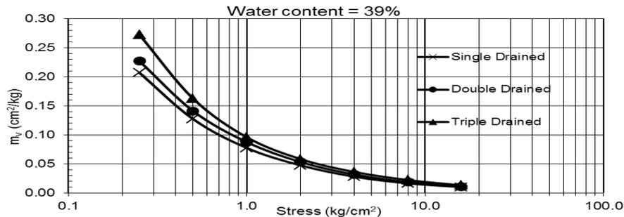
**Fig. 5: Relationship between the coefficient of volume change ( $m_v$ ) and stress for different drainage at water content 39%**
