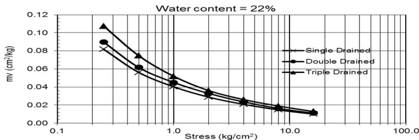
**Fig. 3: Relationship between the coefficient of volume change ( $m_v$ ) and stresses for different drainage at water content 22%**
