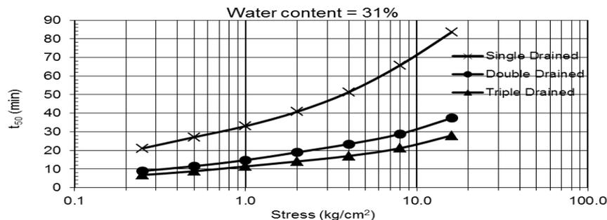
Fig. 14: Relationship between time of consolidation ( $T_{50}$ ) and stresses for different drainage at water content 31%
