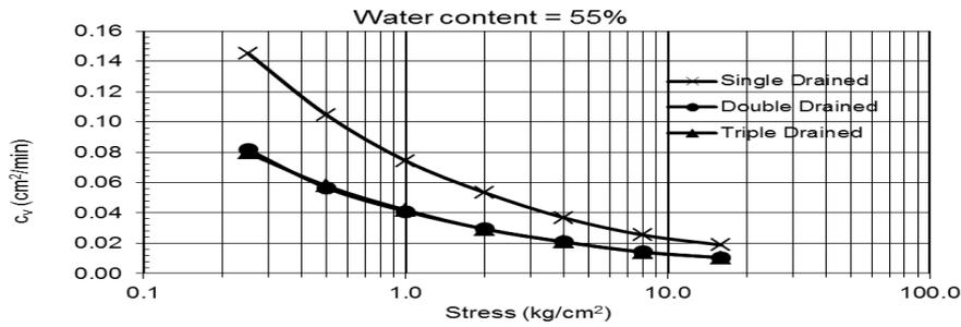
Fig. 12: Relationship between coefficient of consolidation ( $c_v$ ) and stresses for different drainage at water content 55%
