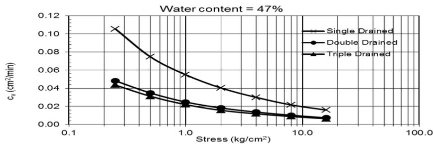
**Fig. 11: Relationship between coefficient of consolidation ( $c_v$ ) and stresses for different drainage at water content 47%**
