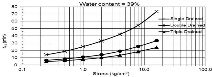
Fig. 15: Relationship between time of consolidation (T<sub>50</sub>) and stresses for different drainage at water content 39%
