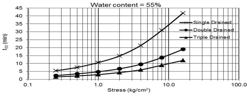
Fig. 17: Relationship between time of consolidation (T<sub>50</sub>) and stresses for different drainage at water content 55%
