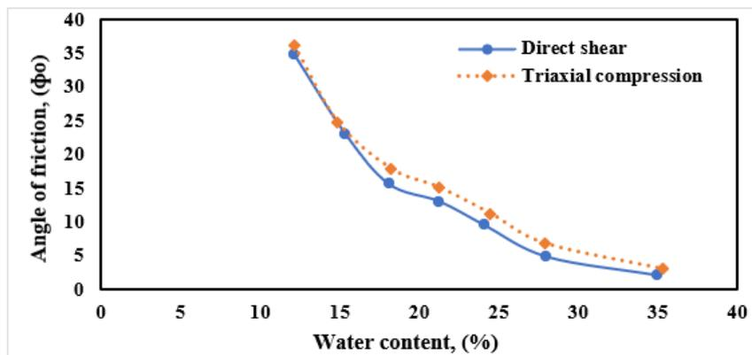
Fig. 8: Comparison between the friction angle in shear and triaxial test at water content from 12.2% to 35%.
