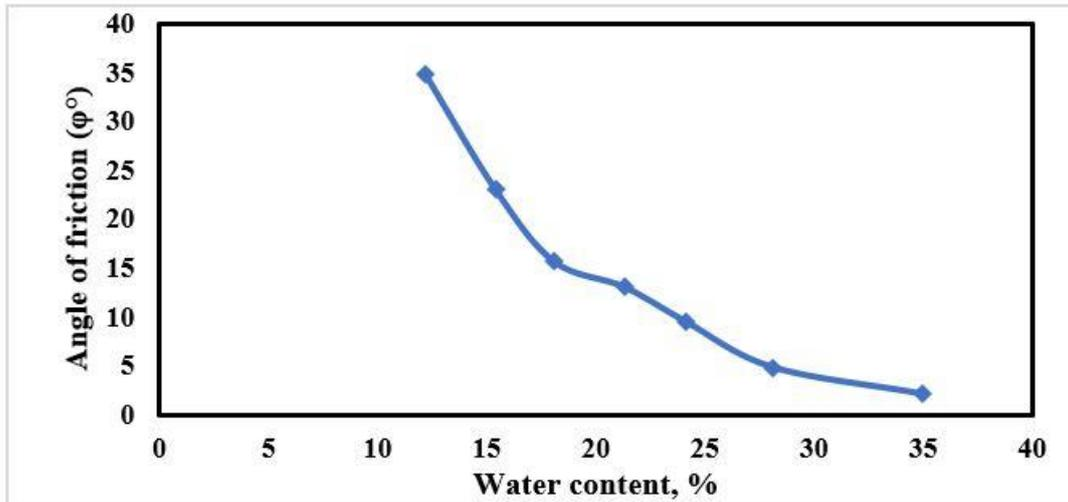
Fig. 2: Relation between friction angle  $\phi$  and water content
