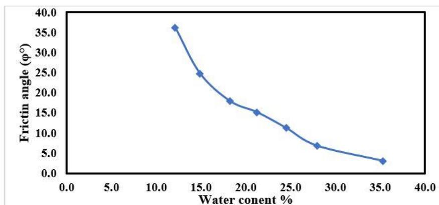
**Fig. 5: relation between the friction angle & the water content %**
