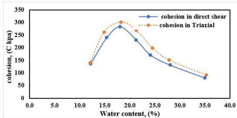
Fig. 7: Comparison between the Cohesion in direct shear and triaxial test at water content from 12.2% to 35%.
