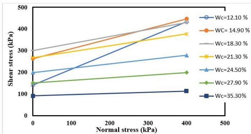
**Fig. 4: Relation between shear stress and normal stress at water content from 12.20% to 35.00%**
