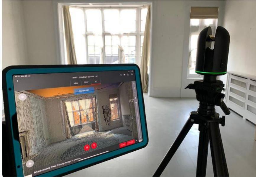
**Figure 4: LeicaBLK laser scanner.**
