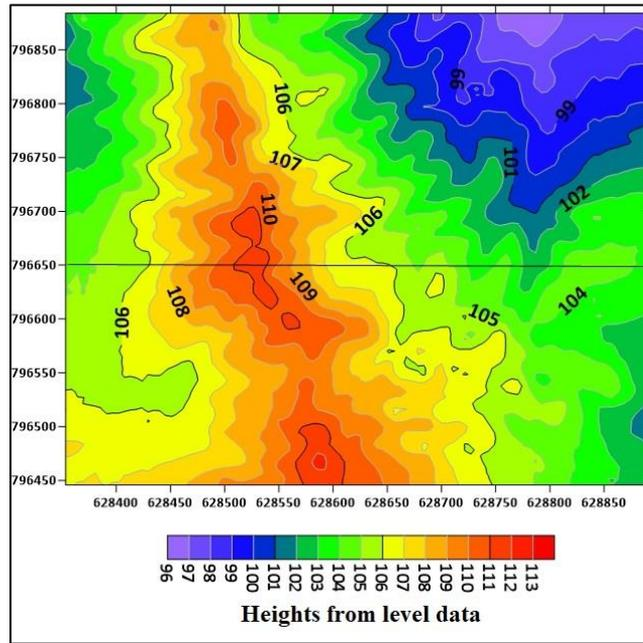
Fig. 4: Contour lines from Level data.
