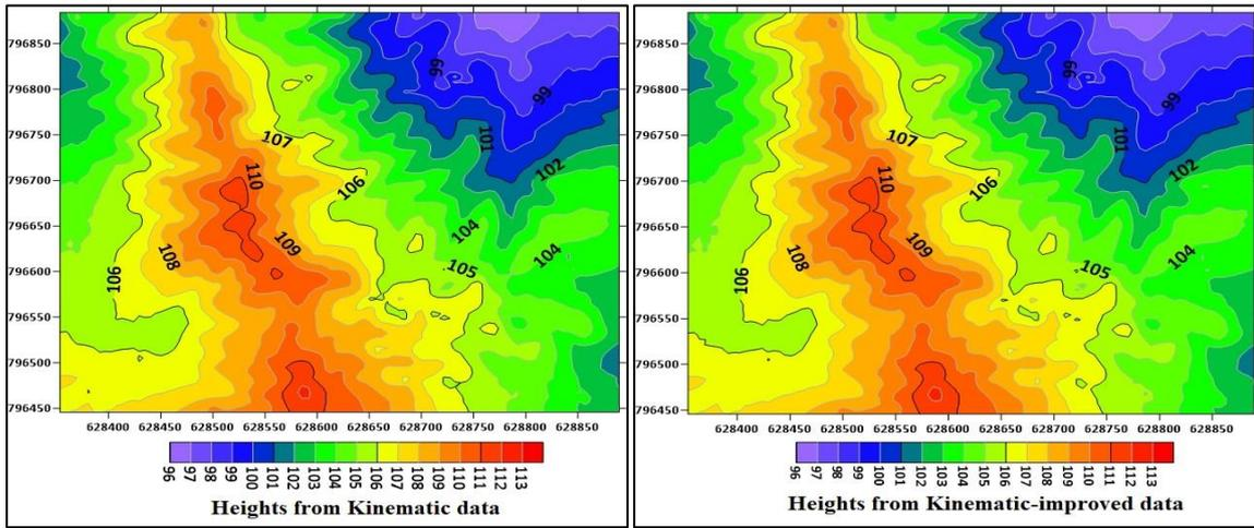
**Fig. 6: Contour lines from kinematic and improved kinematic data.**
