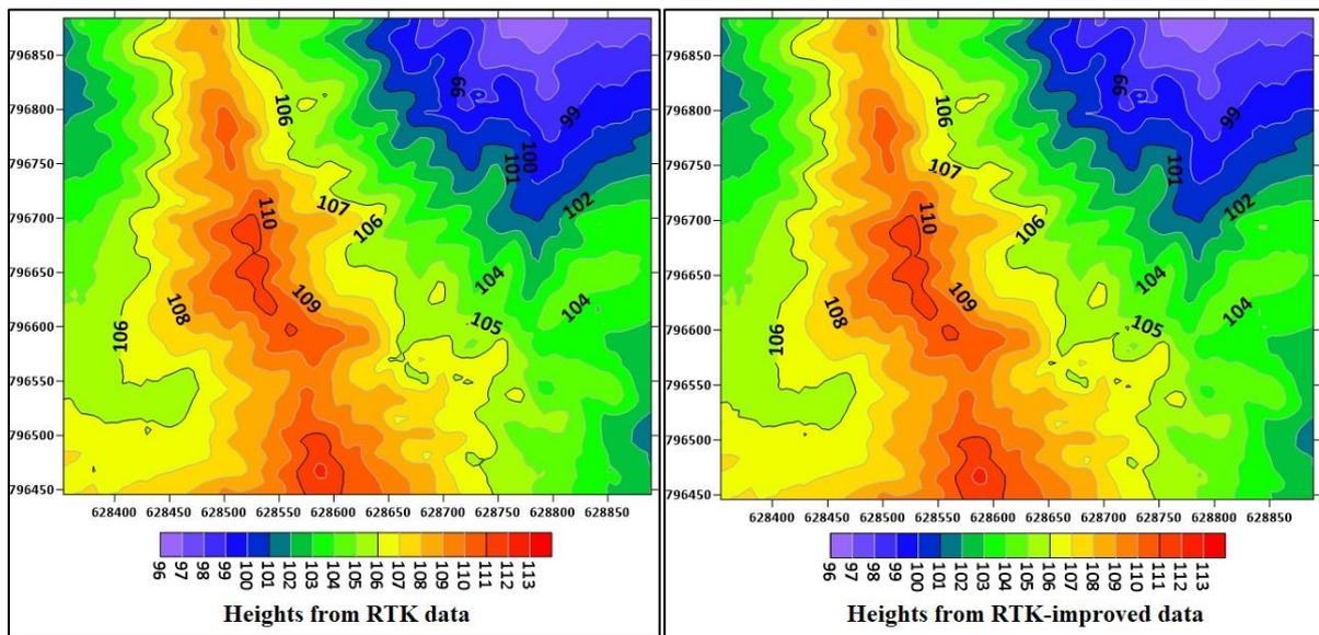
Fig. 5: Contour lines from RTK and improved RTK data.
