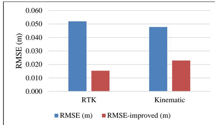
**Fig. 3: RMSE values of the heights from the RTK and kinematic modes pre- and post-improving.**
