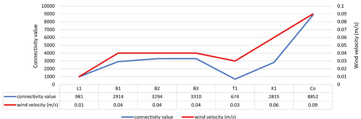
Figure 12: The connectivity value and simulated wind velocity per each room source: Author.
