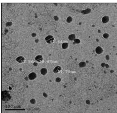
Fig 2: TEM image showing eggshell nanoparticles Characters (magnification x60000), (scale bar 100 nm).
