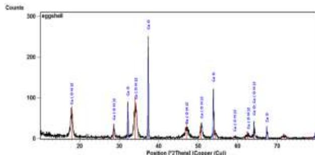
Fig.1: Shows the XRD pattern of eggshell nanoparticles after thermal treatment at 1200 °c and milling
