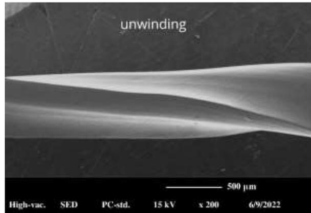
**Figure 1:** Edge file shows unwinding of the flutes after preparing 9 canals in the TAC group.
