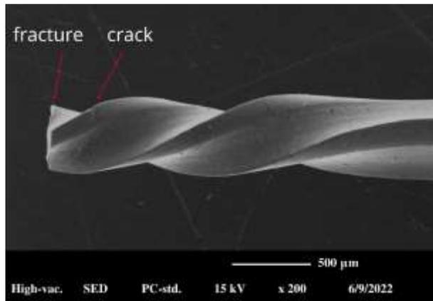
**Figure 2:** Edge file cracks and fractures after preparing 9 canals in the CAC group.
