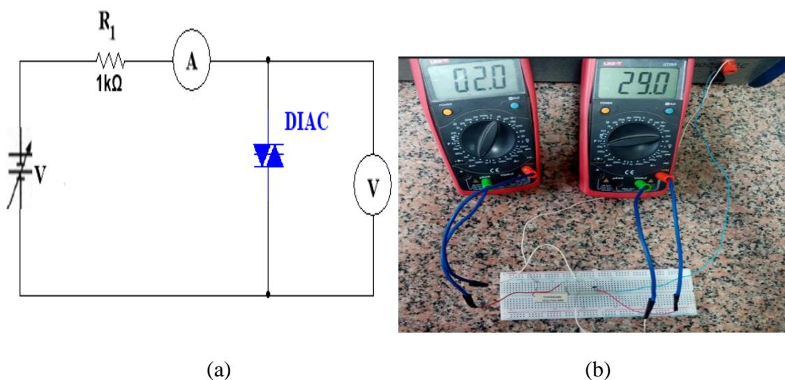
Fig. (4): The characterization circuit of DIAC (a) and its practical implementation (b)
