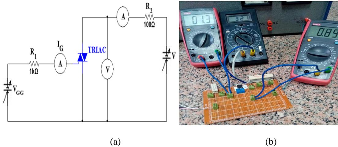
Fig. (3): The characterization circuit of TRIAC (a) and its practical implementation (b)
