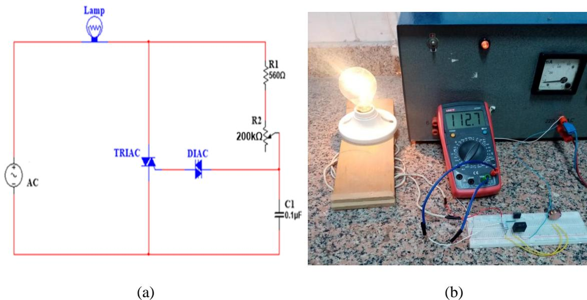
Fig. (5): Schematic illustration showing proposed electronic illumination control circuit (a) and its practical implementation (b)
