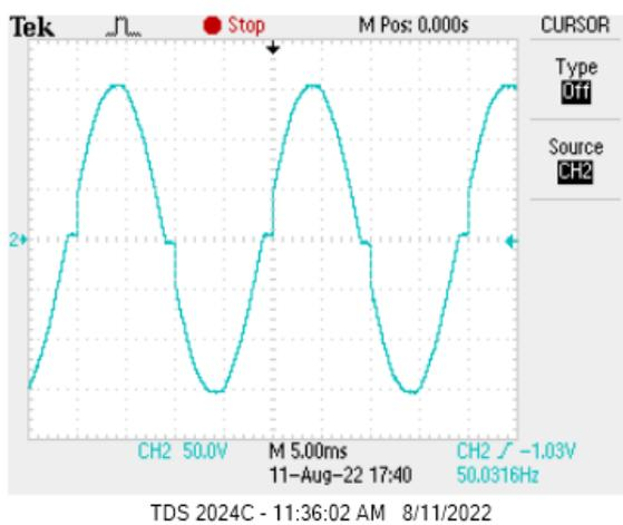
(b)  $\alpha=18^\circ$  at  $R_2 = 1.0 \text{ k}\Omega$
