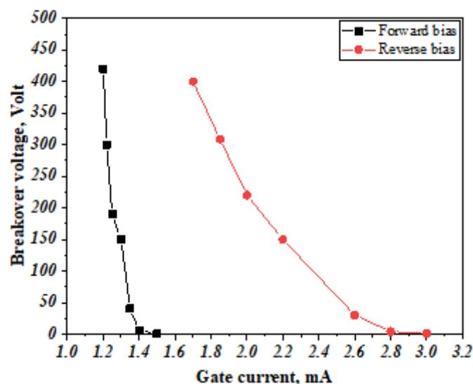
Fig. (7): Dependence of TRIAC break over voltage on its gate current
