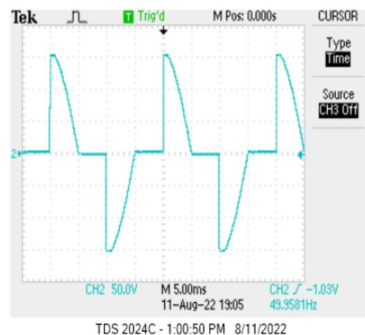
(c)  $\alpha=90^\circ$  at  $R_2 = 110 \text{ k}\Omega$
