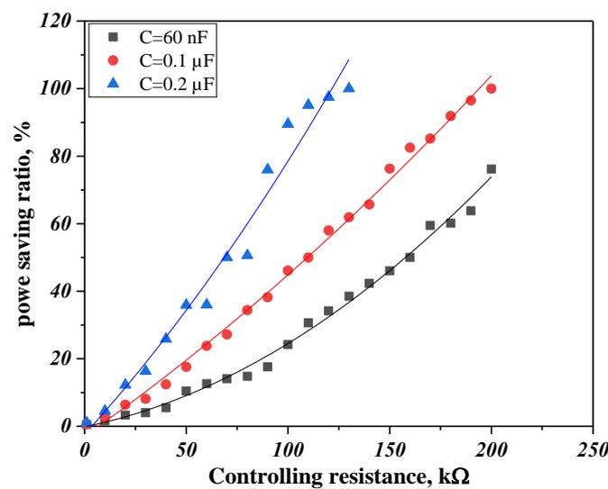
Fig. (12): Dependence of the power saving percentage ratio on the controlling resistance ( $R_2$ ), plotted at different  $C_1$ .
