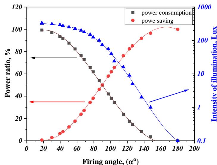
Fig. (11): Effect of firing angle on the intensity of illumination, percent of power consumption and power saving ratio.
