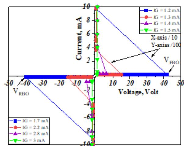
Fig. (6): Static characteristic curves of TRIAC (BT136)
