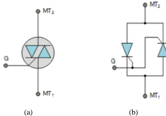
Fig. (1): TRIAC device: (a) electronic symbol, and (b) its equivalent circuit.
