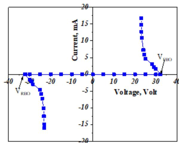
Fig. (8): Static characteristic curves of DIAC (DB3)
