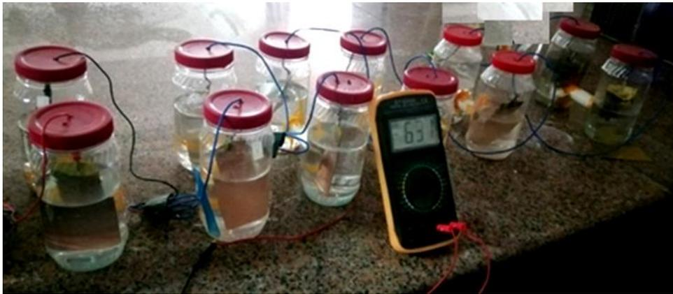
**Fig. (5).** Stacked series 6-MFCs circuit
