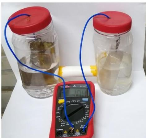
**Fig. (4).** Laboratory scale designed MFC
