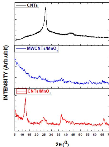
Fig. 3- XRD analysis of the synthesized nanocomposites.
