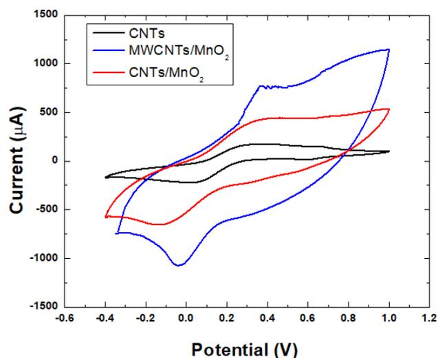
**Fig .7- CV of prepared nanocomposites at scan rate**
