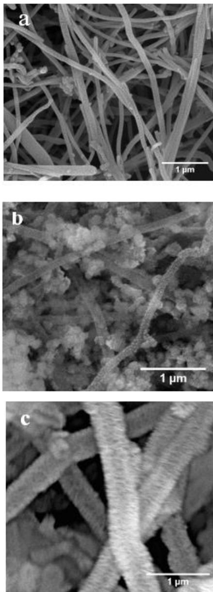
Fig. 5-SEM images of (a)CNTs ; (b) MWCNTs/MnO<sub>2</sub> ; (C) CNTs/MnO<sub>2</sub>
