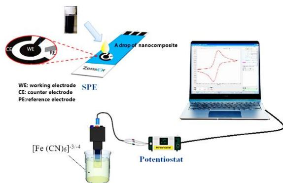
**Fig.6-Steps of working electrode modification with the prepared nanocomposites**
