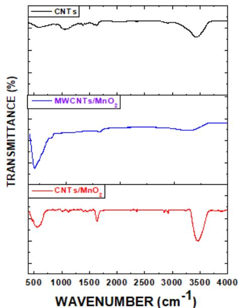
Fig.4- FTIR spectrum of CNTs, MWCNTs/MnO<sub>2</sub> and CNTs/ MnO<sub>2</sub>.
