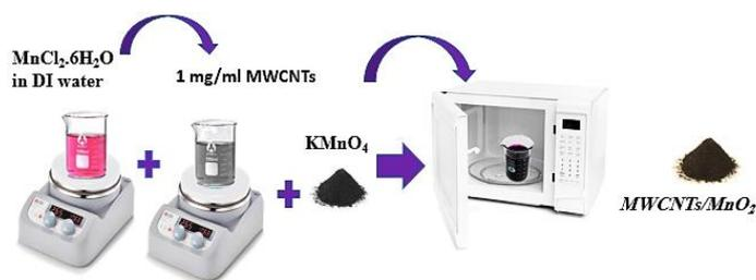
Fig. 1- Illustration of the microwave preparation method.
