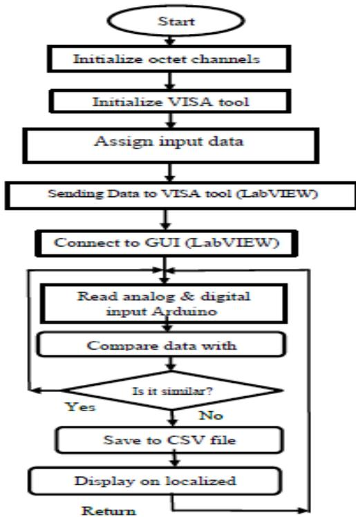
Figure 4 : system operation flow
