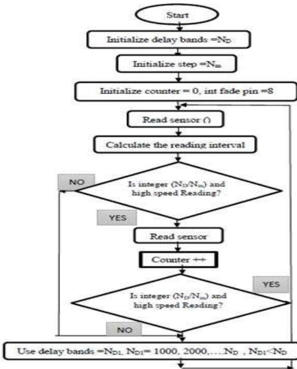
Figure 5: Saving system flow chart
