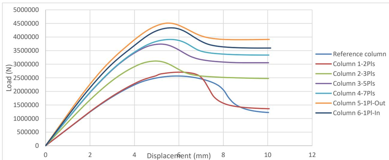
Figure 15. The load-displacement curve for all columns.
