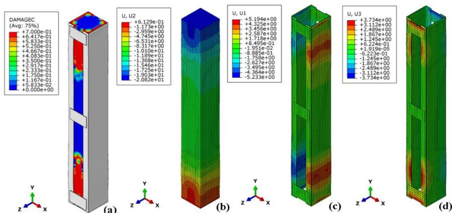
Figure 10. The damage of column 2-3PIs and the displacements in the column and the steel cage.
