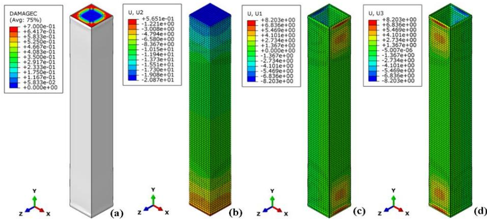
Figure 14. The damage of column 6-1PI-In and the displacements in the column and the steel cage.
