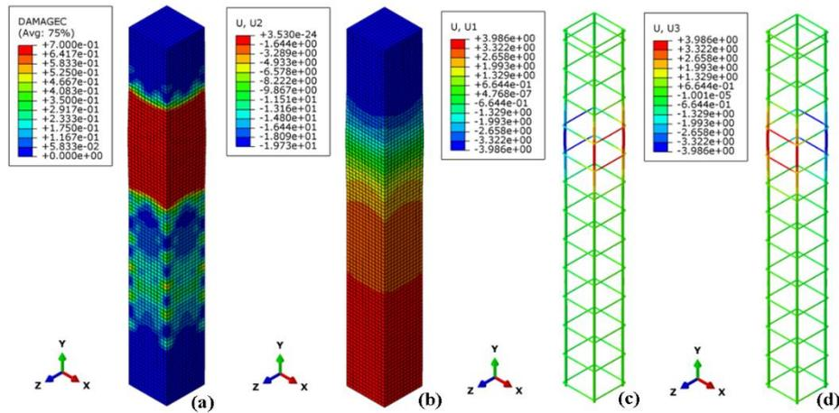
Figure 8. The damage of the reference column and the displacements in the column and the reinforcement steel.
