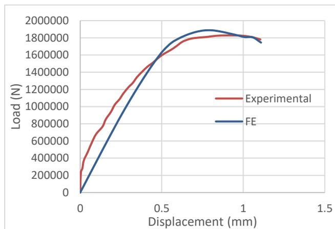
Figure 7. The load-displacement curve of the experimental and FE model of the second column.
