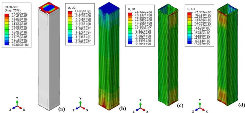
Figure 13. The damage of column 5-1PI-Out and the displacements in the column and the steel cage.
