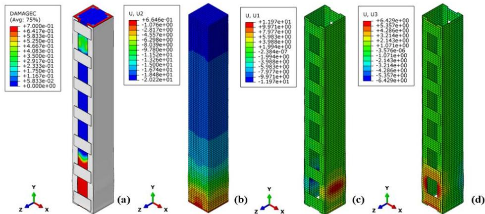
Figure 12. The damage of column 4-7PIs and the displacements in the column and the steel cage.
