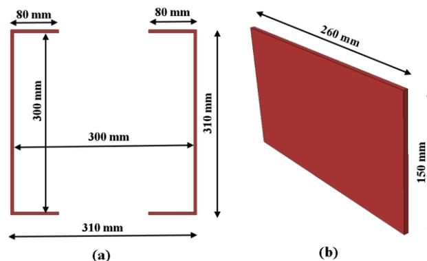
Figure 2. (a) Details of the two C-channels steel cage; (b) The connecting Batten plate.
