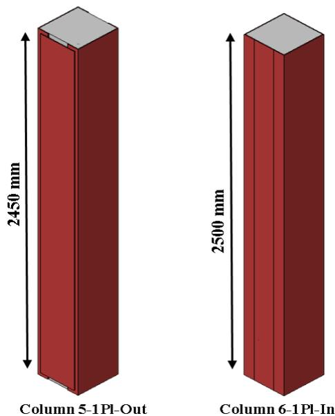
Figure 4. The second group of strengthened columns.
