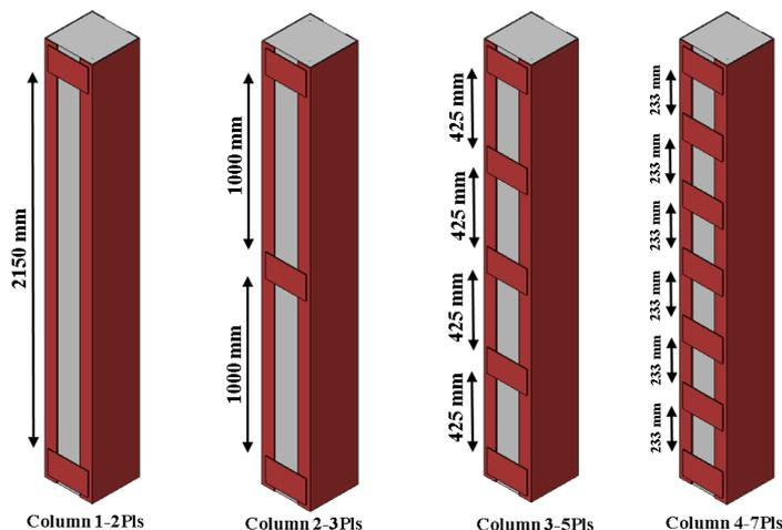
Figure 3. The first group of strengthened columns.
