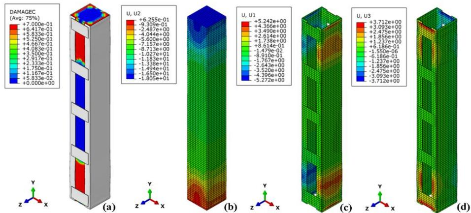
Figure 11. The damage of column 3-5PIs and the displacements in the column and the steel cage.
