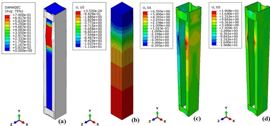
Figure 9. The damage of column 1-2PIs and the displacements in the column and the steel cage.
