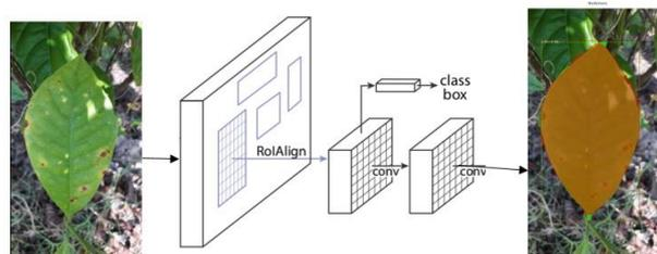
**Figure 2.** Framework of the proposed Mask RCNN, Johnson, J. W. (2018).
