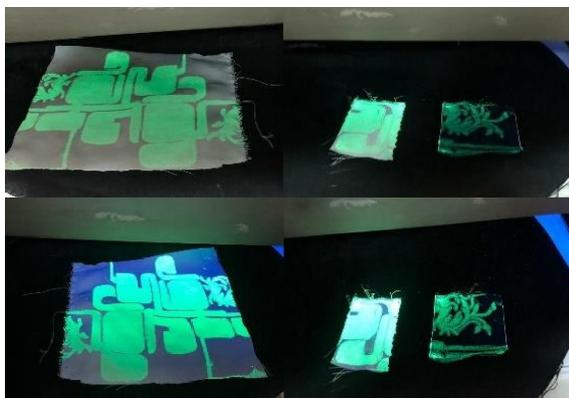
**Fig.3. Images of photochromic dyes on the surfaces of polyester fabric that is treated with silicone rubber polymer and TiO<sub>2</sub> NPs.**
