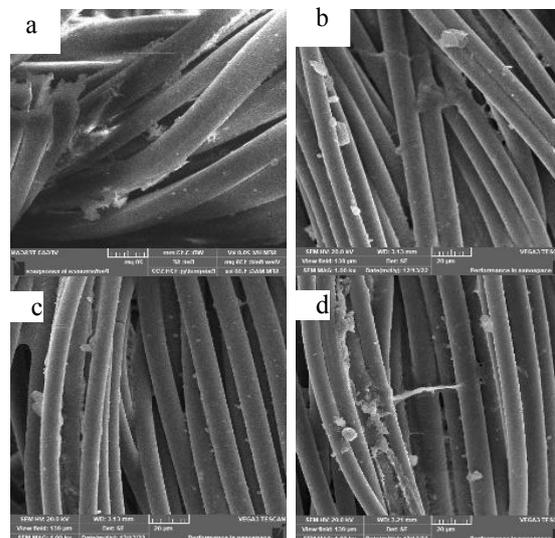
**Fig.1. SEM images of the treated polyester fabric with silicone rubber and  $\text{TiO}_2$  NPs (3%)**
