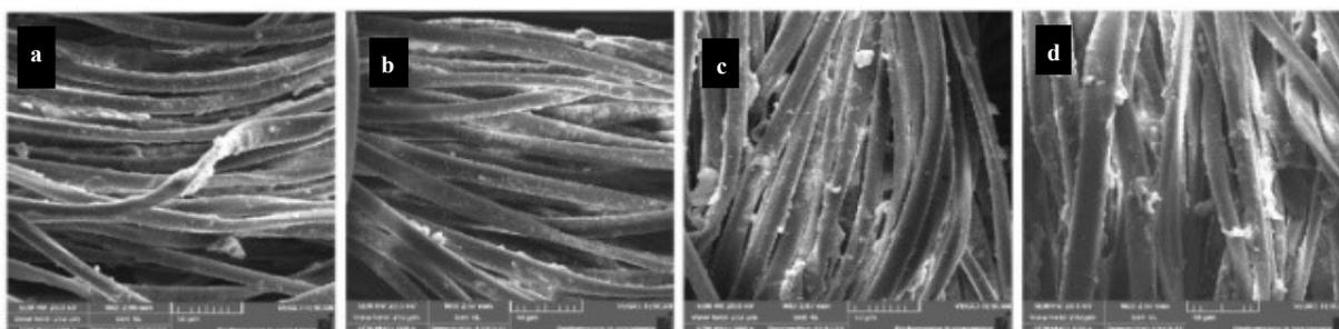
**Fig.1.** SEM images of treated polyester fabrics with ZnO(a,b). images of treated cotton fabrics with silicone rubber (c,d)
