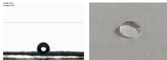
**Figure 2.** Cotton/polyester blended fabrics treated by PFHMA.
