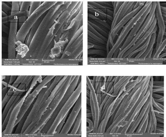
**Figure 1.** SEM images of treated pure cotton fabrics.
