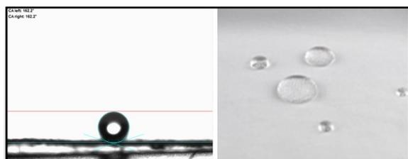
Figure 3 contact angle of treated cotton fabric using 3% of silicon /chitosan.
