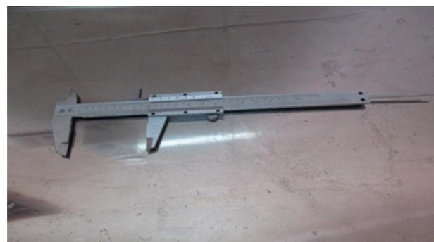
**Figure 2** Vernier caliper gauge.
