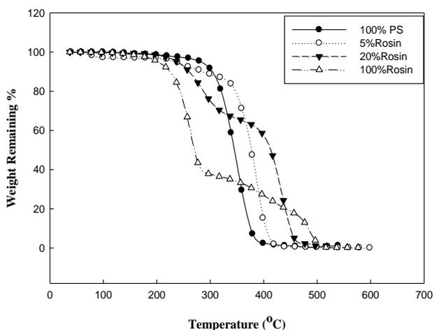
**Fig. (4):** TGA thermogram of unirradiated PS and its blends (PS/ rosin) at various compositions
