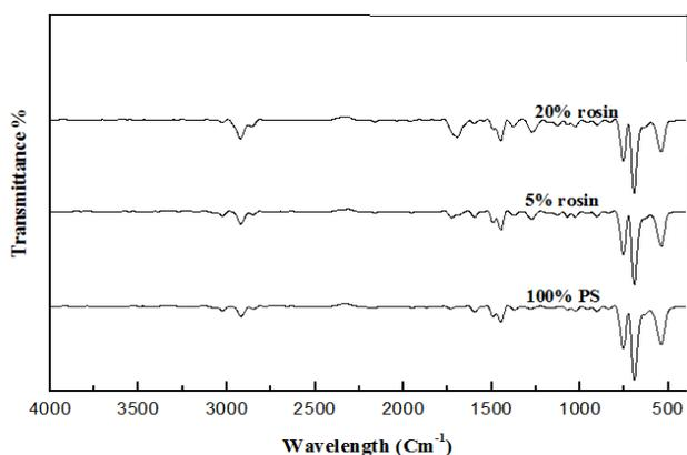
**Fig. (11): IR spectra of PS and its blends (PS/ rosin) at various compositions irradiated to 100kGy**
