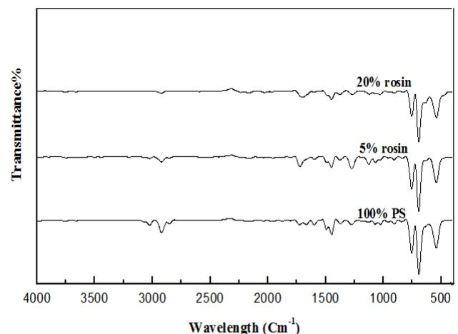
**Fig. (12): IR spectra of PS and its blends (PS/ rosin) at various compositions irradiated to 200kGy**
