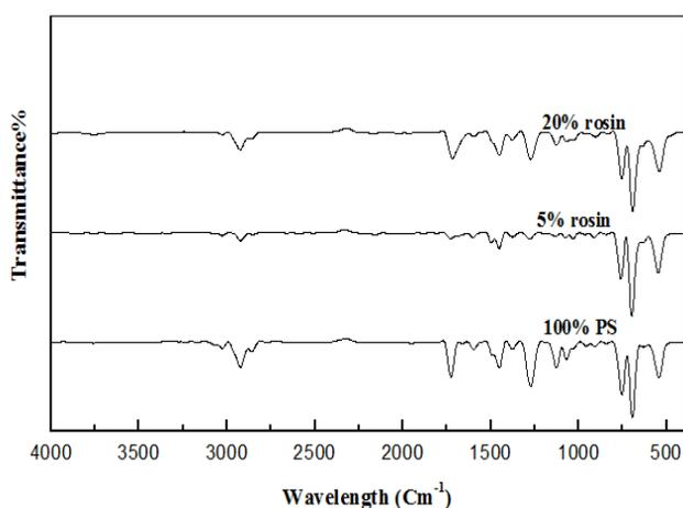
**Fig. (10): IR spectra of unirradiated PS and its blends (PS/ rosin) at various compositions**
