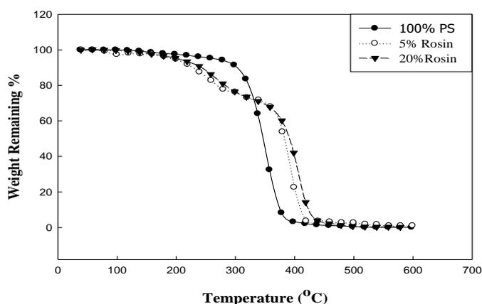
**Fig. (6):** TGA thermogram of PS and its blends (PS/ rosin) at various compositions irradiated at 200 kGy
