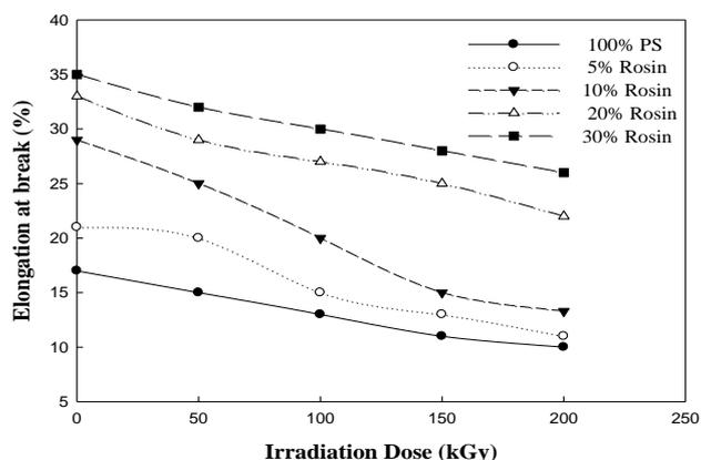
Fig. (3): Effect of irradiation dose on the  $E_b$ % of PS and its blends (PS/ rosin) at various compositions
