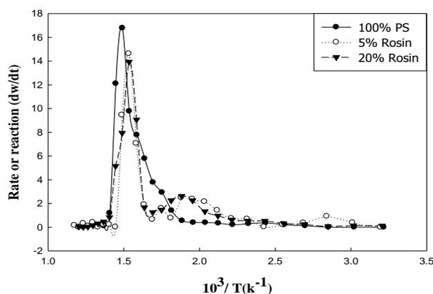
**Fig. (9):** Rate of reaction ( $dw/dt$ ) of PS and its blends (PS/ rosin) at various compositions irradiated at 200 kGy
