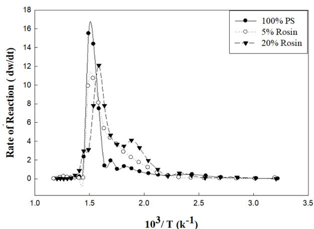
**Fig. (8):** Rate of reaction ( $dw/dt$ ) of PS and its blends (PS/ rosin) at various compositions irradiated at 100 kGy
