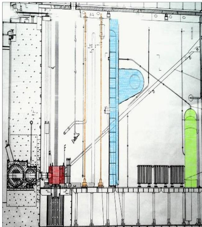
Fig. (1.b): Vertical cross section of the reactor pool
