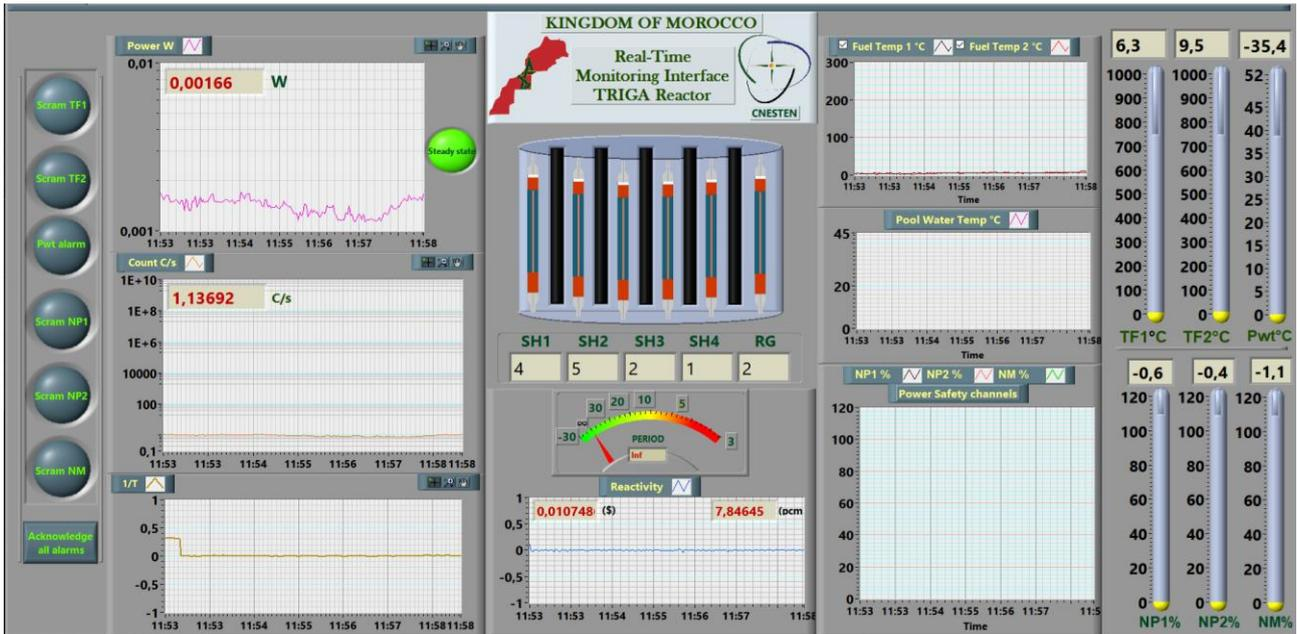
Fig. (3): Live Data Screen with all necessary data to perform the experiments
