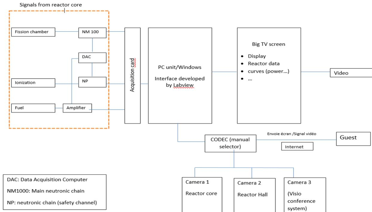
**Fig. (5): Schematic representation of the capabilities of the system, which transmits two video signals from the reactor control room to the guest institution's classroom**
