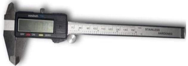
Figure (1): Digital Vernier caliper
