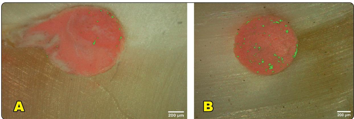
Fig. (1) Stere-photomicroscopic imaging: A) voids in continuous wave technique B) Voids in lateral condensation technique
