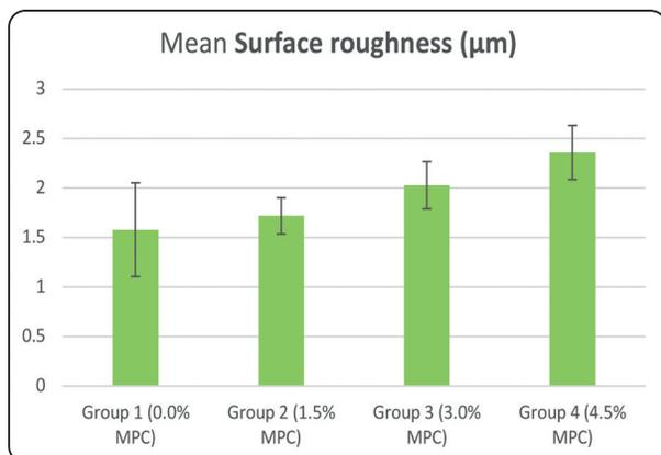
Fig. (7) Bar graph showing the means and standard deviations of surface roughness ( $\mu\text{m}$ ) for the tested groups.
