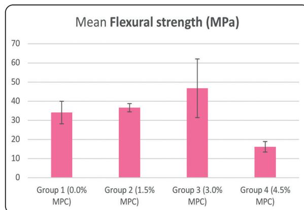
Fig. (8) Bar graph demonstrating the means and standard deviations of flexural strength (MPa) for the tested groups.
