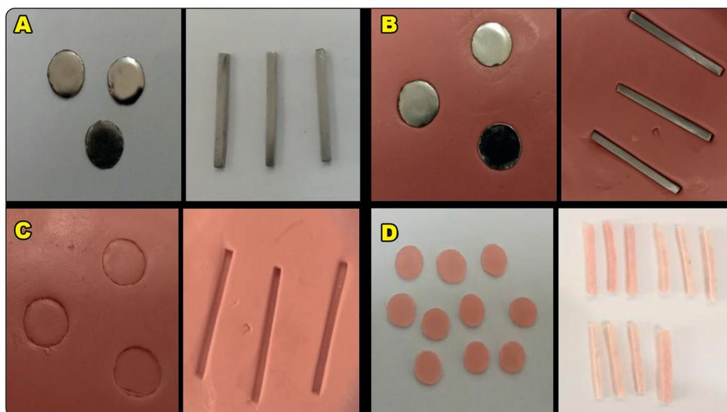
Fig. (1) Steps of preparation of the acrylic sample (A) Stainless steel molds with various dimensions for each test (B) Using stainless steel mold in rubber base to make space with similar dimensions, (C) Space for self-cure acrylic insertion, (D) Acrylic specimens of different dimensions utilized in this study.
