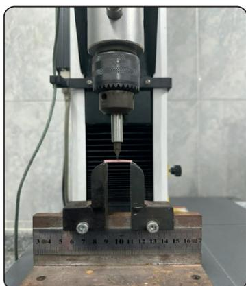
Fig. (4) Specimen mounted on Universal Testing Machine for three-point flexure test.
