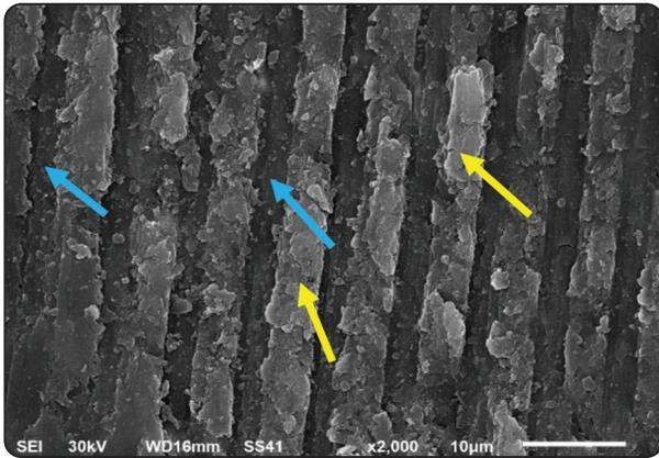
Fig. (14) L.S. of dentinal tubules after 15 days of treatment with chitosan
