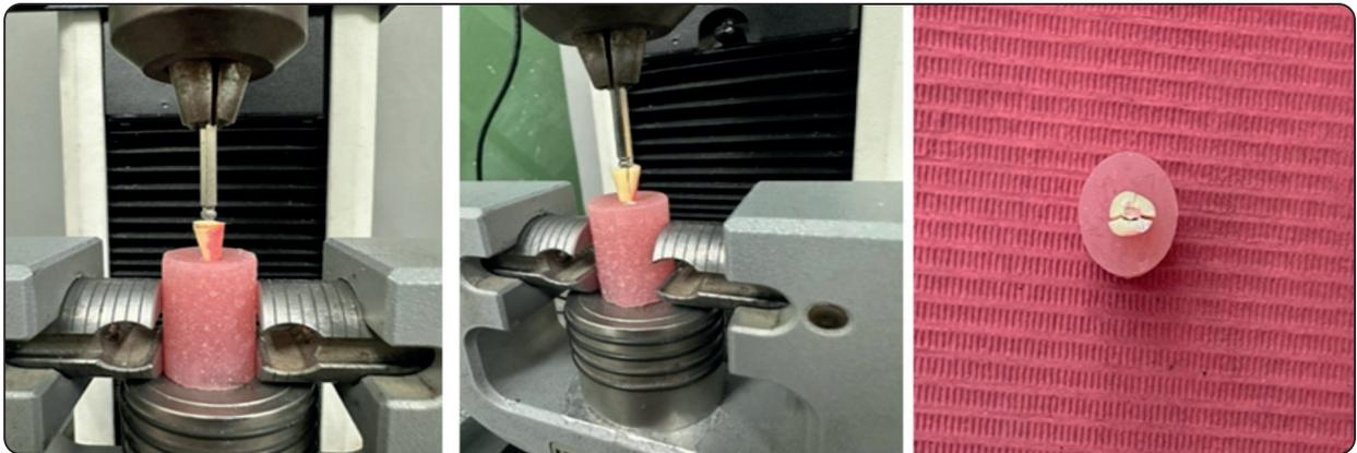
Fig. (1) Sample fracture after vertical loading with the Universal testing machine.
