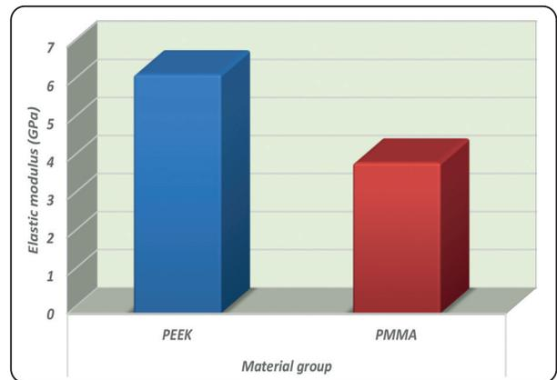
Fig. (2) Column chart comparing the mean scores Elastic Modulus of each group.
