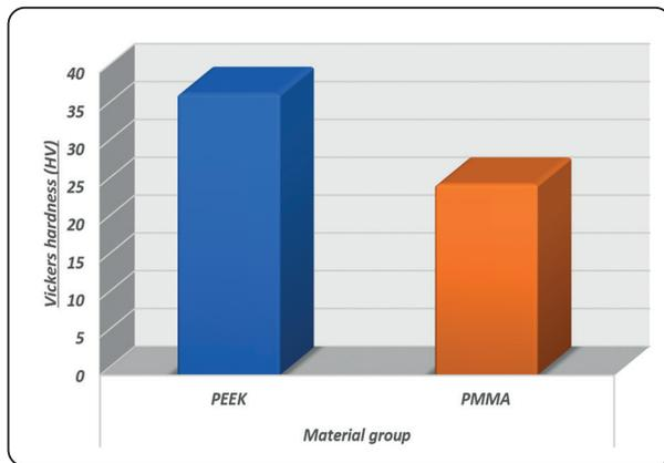
Fig (1) Column chart comparing the mean scores Vickers hardness of each group.
