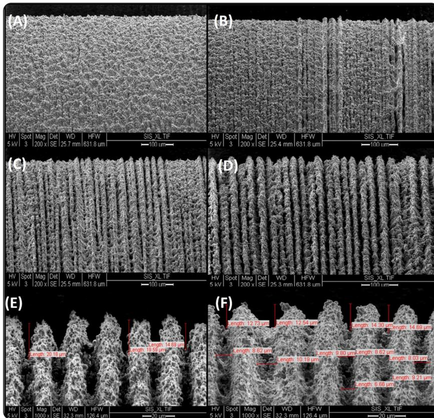
Fig. (3) SEM images with linear measurements recorded. A: Rod #1 zone 1. B: Rod #2, zone 5. C: Rod #2, zone 6. D: Rod #2, zone 11. E: Rod #2, zone 12. F: Rod #3, zone 14.
