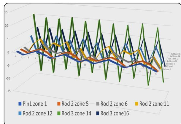
Fig. (5): Surface topography profilometry of titanium rods different laser micro-grooving zones
