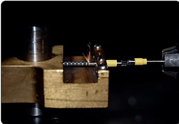
Fig. (1) Titanium rod laser micro-grooving set-up
