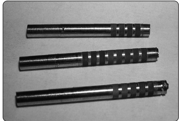
Fig. (2) The titanium alloy laser engraved rods.
