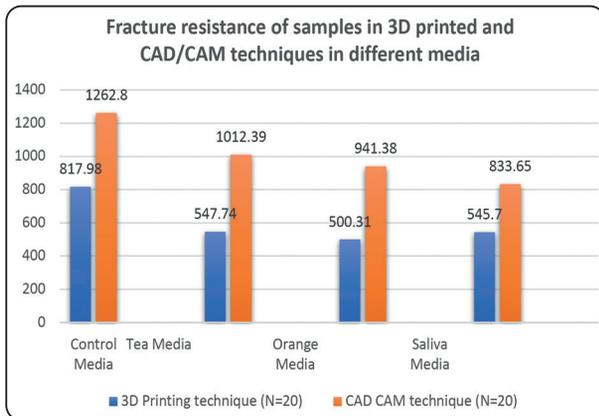
Fig. (4) Comparison of fracture resistance of samples in 3D printed technique and CAD/CAM techniques in different sub groups
