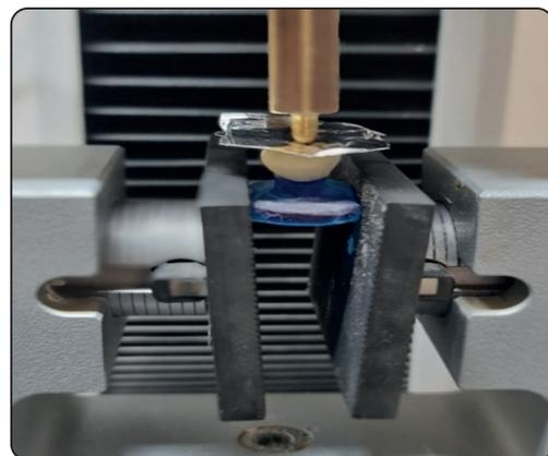
Fig. (3) measurement of fracture resistance of the sample
