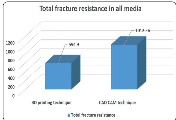
Figure (5) Total fracture resistance in all media
