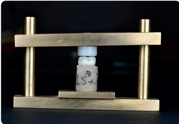
Fig. (2) Specially designed copper device used to stabilize the table- top to its corresponding preparation with a constant load of 50 N for 5 minute.
