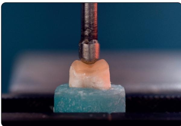
Fig. (2) Steel rod with a round tip used in fracture test
