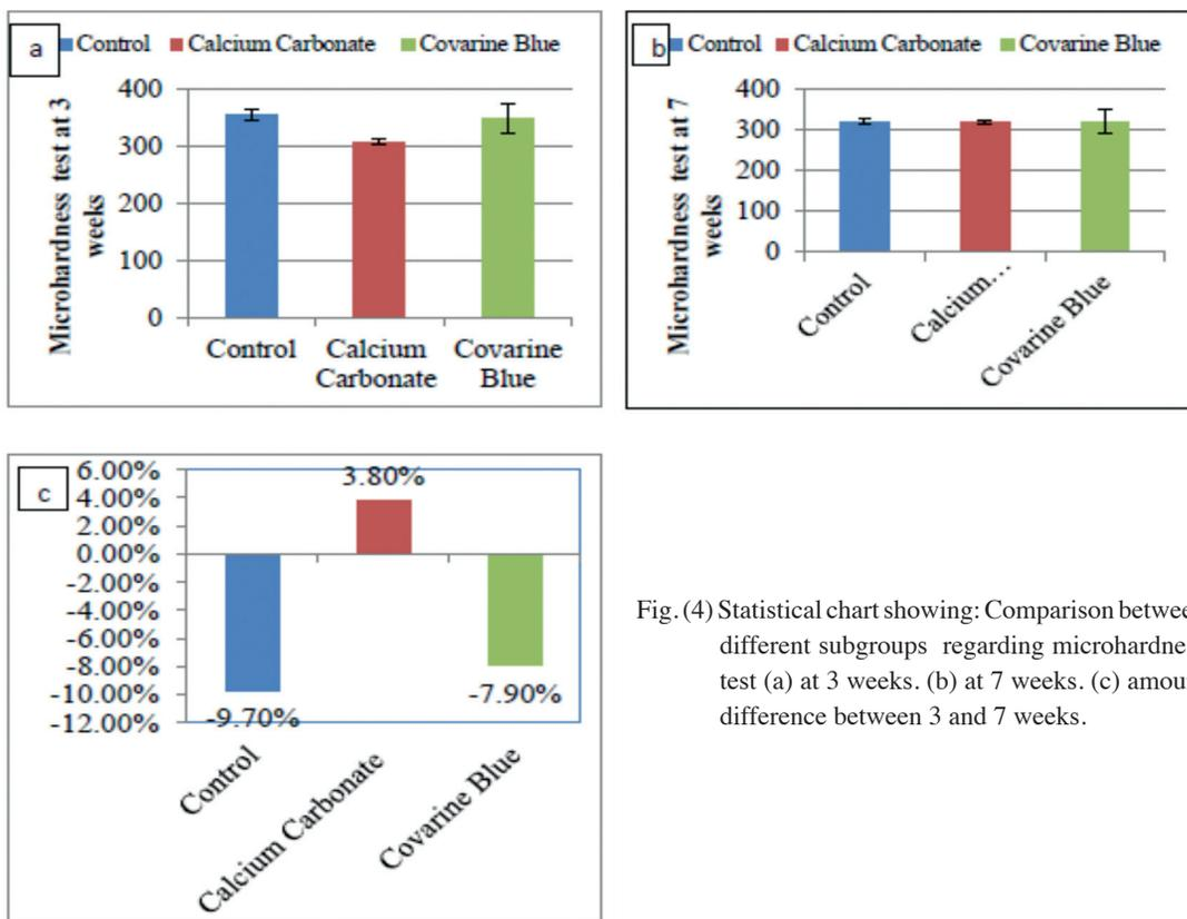
Fig. (4) Statistical chart showing: Comparison between different subgroups regarding microhardness test (a) at 3 weeks. (b) at 7 weeks. (c) amount difference between 3 and 7 weeks.
