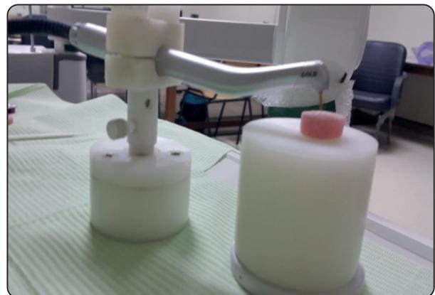
Fig. (2) Custom made plastic assembly used to fix the LASER hand piece
