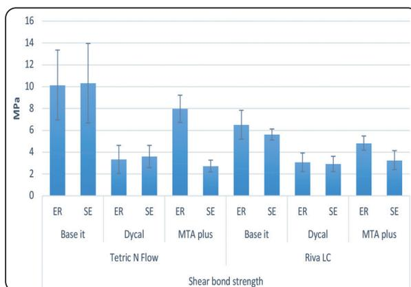
Fig. (1) Bar chart showing mean and standard deviation values (error bars) of shear bond strength for different variables
