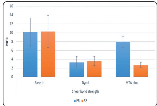
Fig. (3) Bar chart showing mean and standard deviation values (error bars) of shear bond strength within Tetric N flow (B)
