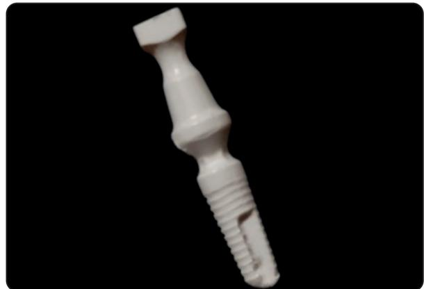
Fig. (4) Milled PEEK implant.
