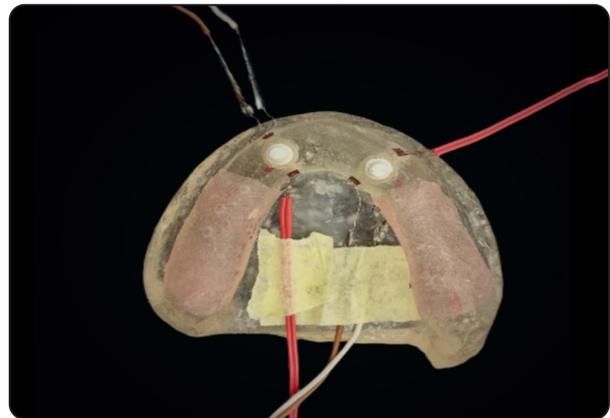
Fig. (6) Strain gauge fixation
