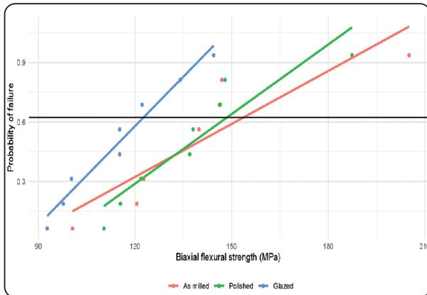
Fig. (3) Probability of failure plot of biaxial flexural strength data.
