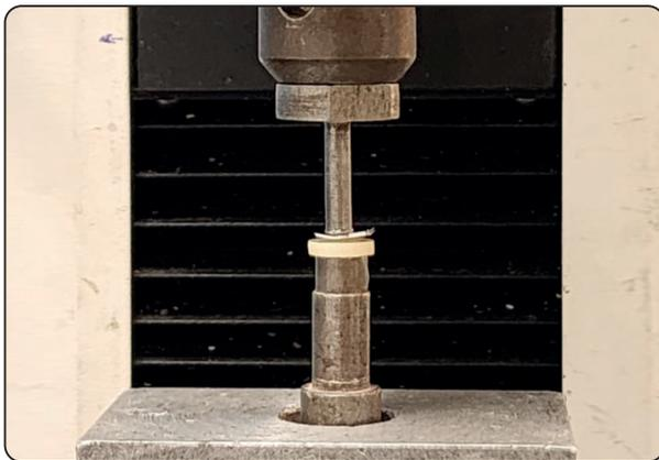
Fig. (1): Biaxial flexural strength test.
