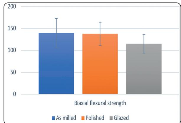
Fig. (2): Bar chart showing mean and standard deviation values (error bars) of biaxial flexural strength for different groups.
