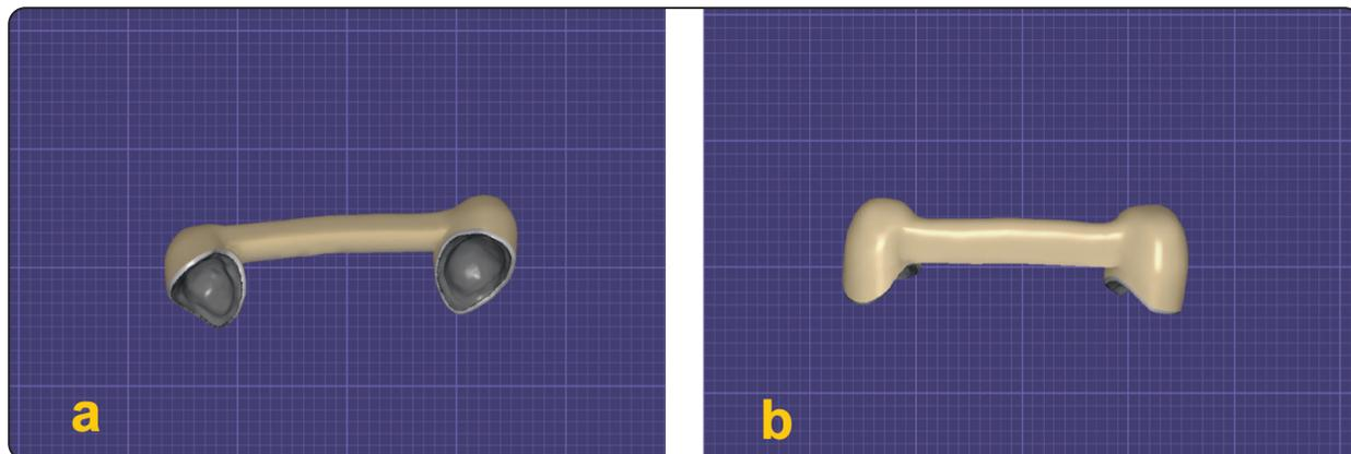
Fig. (1a&b): Digital designing for the bar on virtual model.
