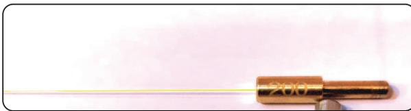
A fiber optic of 200 µm diameter
