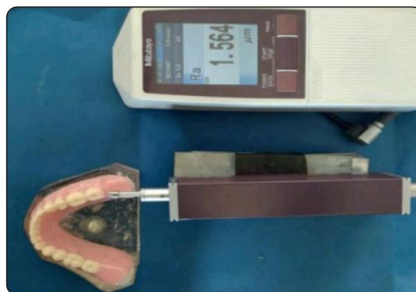
Fig. (8) Measuring the surface roughness for the acrylic dentures modified by Salinized Tio2 Nps)
