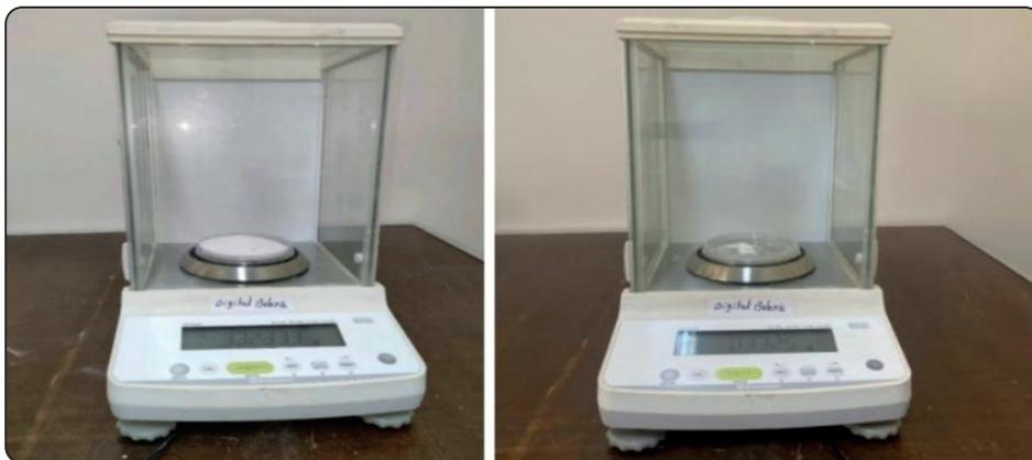
Fig. (4) (Measuring the powder of PMMA and Salinized Tio2 Nps using Digital Balance)
