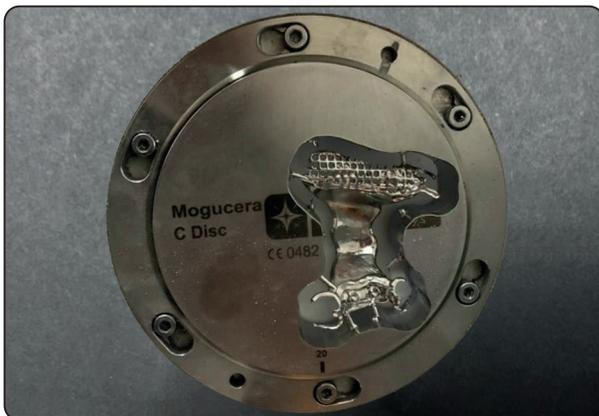
Fig. (3) Milled framework from polished surface
