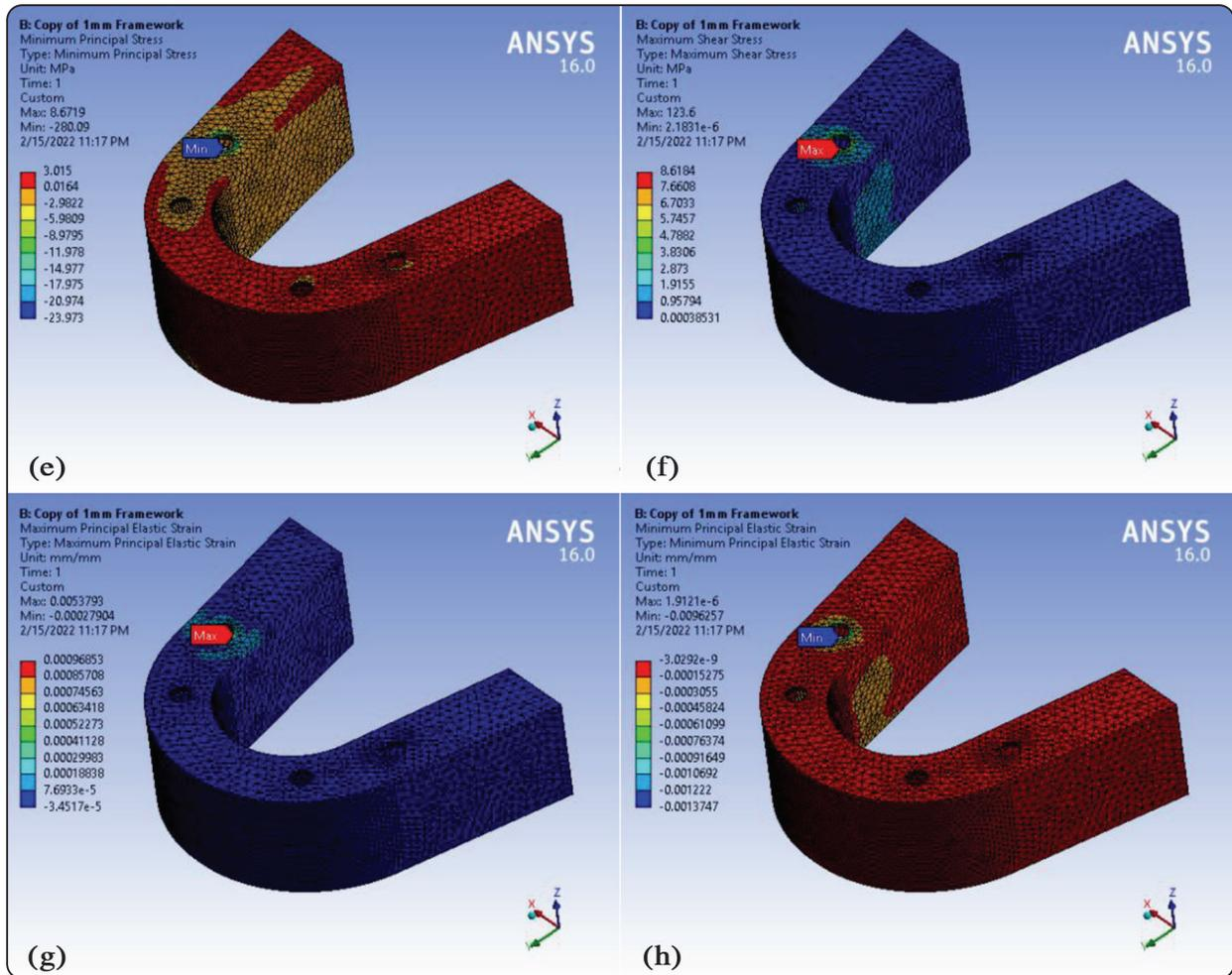
Fig. (2) Max principal stress, (e) Min principal stress, (f) shear stress, (g) Max tensile strain, and (h) Min compressive strain.
