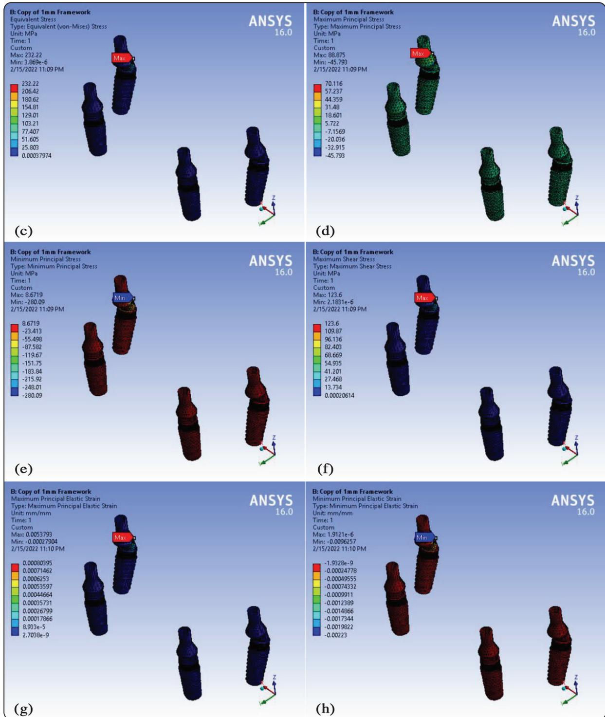
Fig. (3) (c) Von Mises stress, (d) Max principal stress, (e) Min principal stress, (f) shear stress, (g) Max tensile strain, and (h) Min compressive strain.
