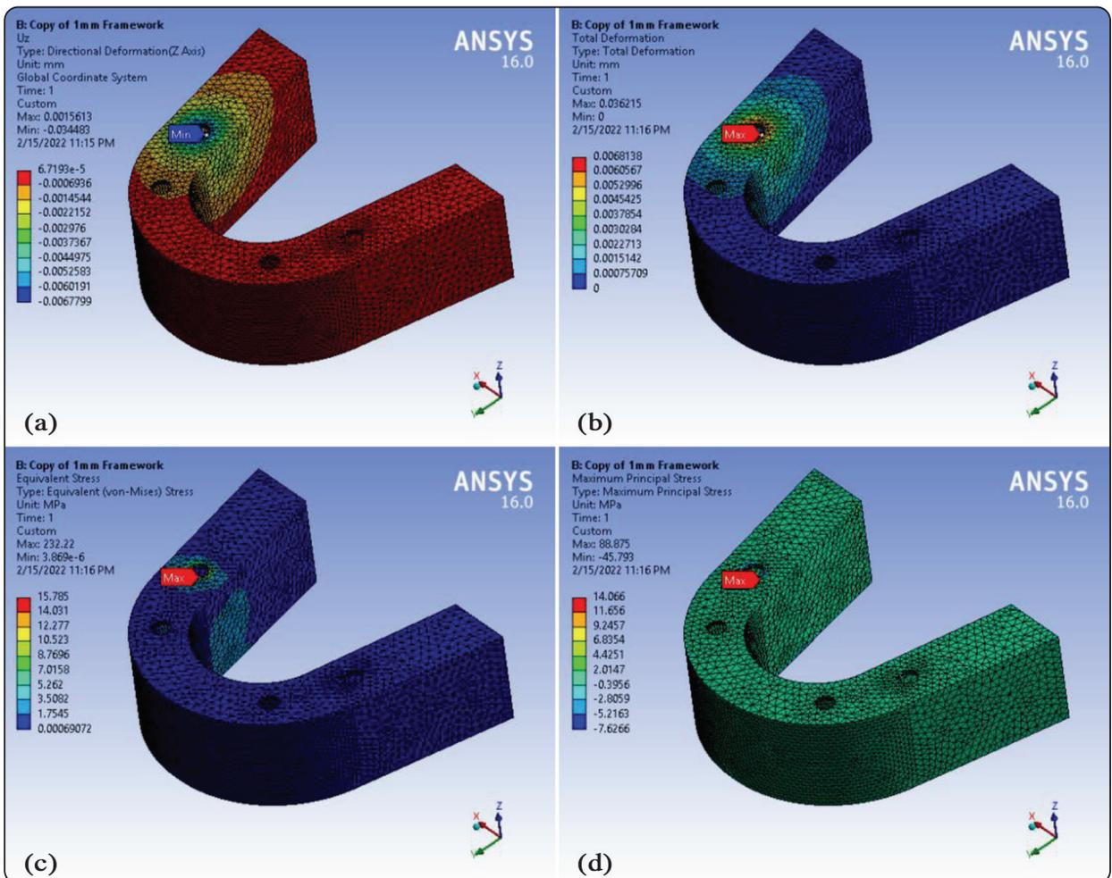
Fig. (2) Cortical bone results; (a) vertical deformation, (b) total deformation, (c) Von Mises stress,
