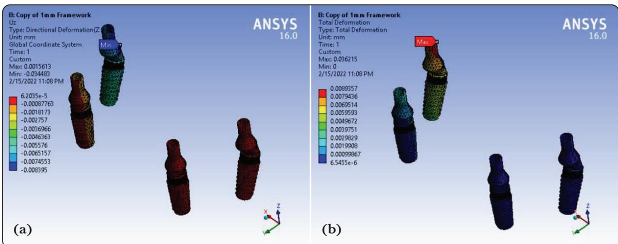
Fig. (3) Implant system results; (a) vertical deformation, (b) total deformation,
