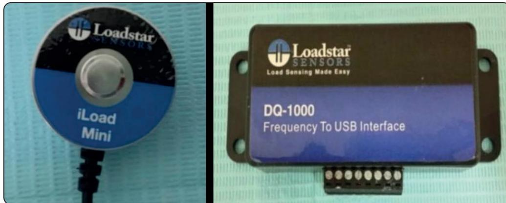
Fig (4): The I-load star sensor device.
